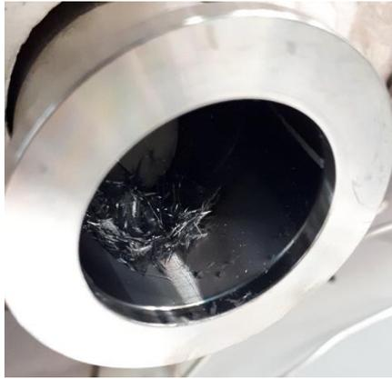
**Figure 6:** View of the crystals formed by the tellurium inside the junction connecting the two furnaces.
