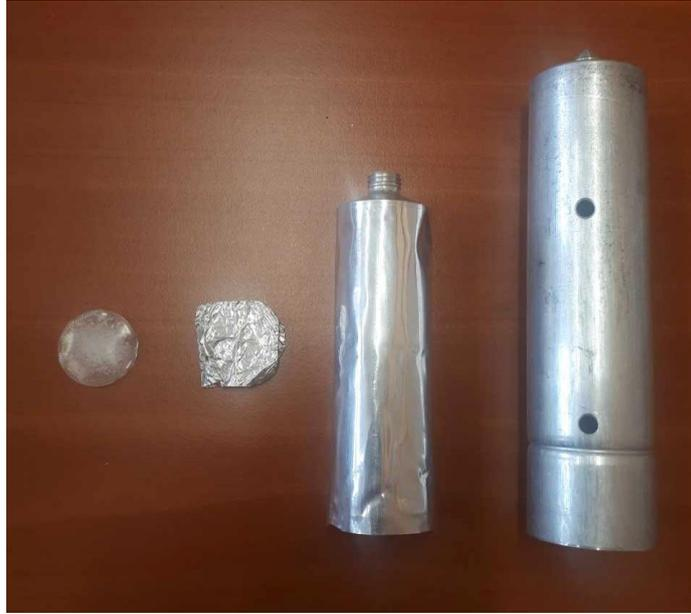
**Figure 2:** Package for neutron irradiation. The filter sample is folded and packaged into the polyethylene, folded into aluminum foil, then stacked into the smaller cylinder. The small cylinder is then loaded into the large one, and the package is sent via a pneumatic delivery system into the reactor.
