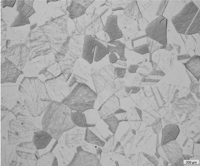
**Figure 24.** Optical micrograph of the etched copper sample, direction 1 (main surface to be studied).
