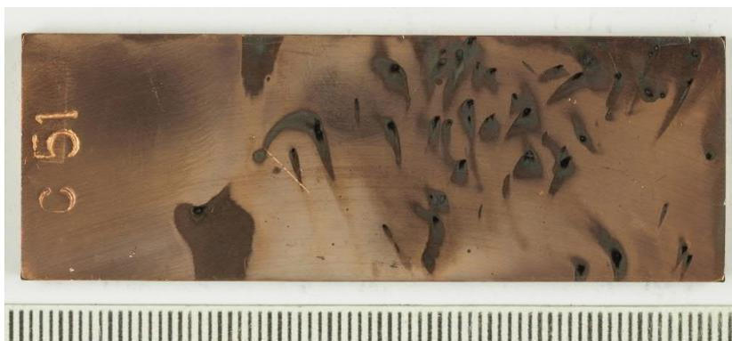
**Figure 11.** Ground sample after four month exposure in solution with sulphide addition of 32 mg/L. Gaps in scale bar 1 mm.
