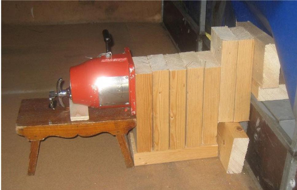
Fig 3.9 Collimated source geometry. Wooden blocks (1 - 10 blocks, 45 - 450 mm) were used as shielding material in front of the collimated Cs-137 source, in this picture with 8 blocks.
