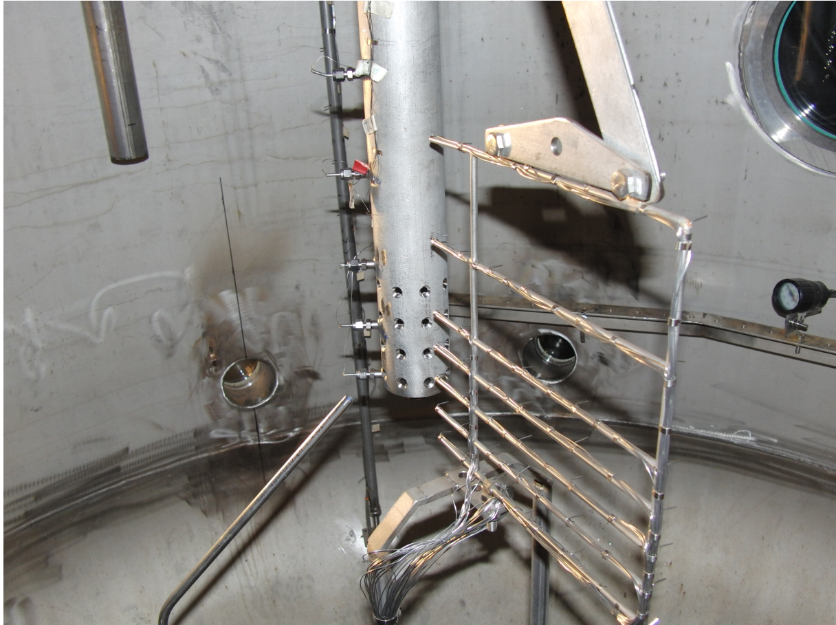
Figure 2. Injection pipe and temperature rake. Only the bottom row of holes is open during the experiment SPA-T1. Picture Markku Puustinen, LUT.
