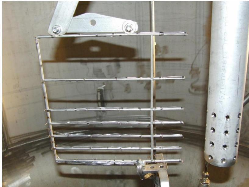
Figure 3. Grid of thermocouples close to the head of the sparger pipe.
