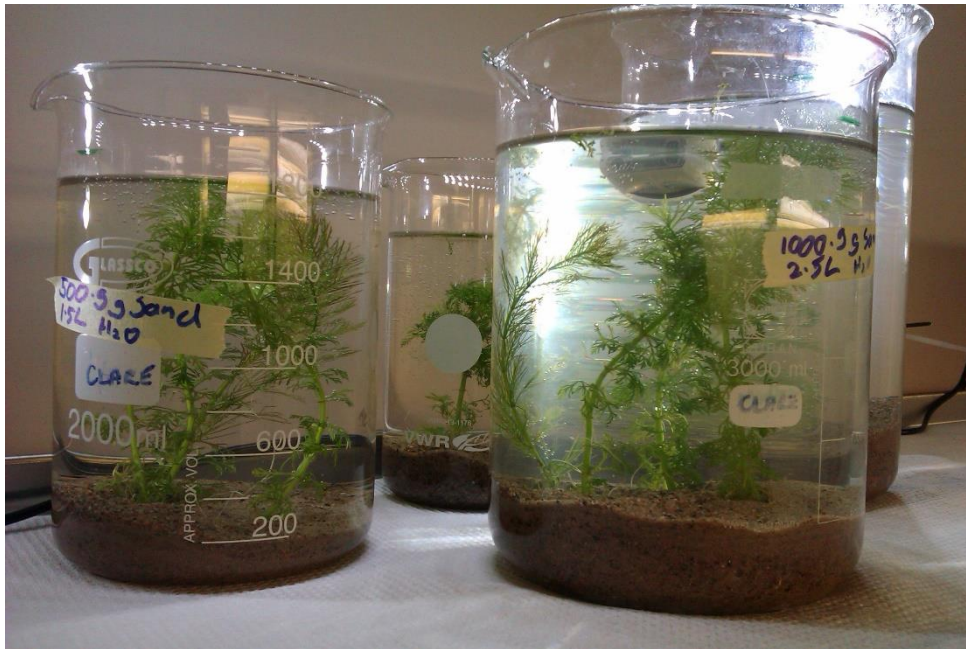
Figure 3. Pre-testing 2L microcosm trials with sediment, freshwater and aquatic plants at Stockholm University.
