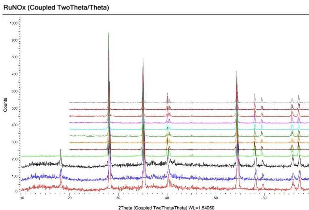
Figure 6. The obtained XRD spectra from the samples of experiments 1 to 12. The height of the peaks was scaled in order to fit in the figure.
