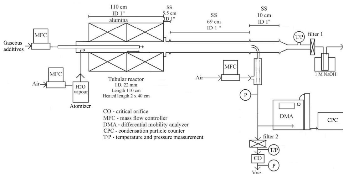
Figure 2. Schematics of the experimental facility for ruthenium transport studies.
