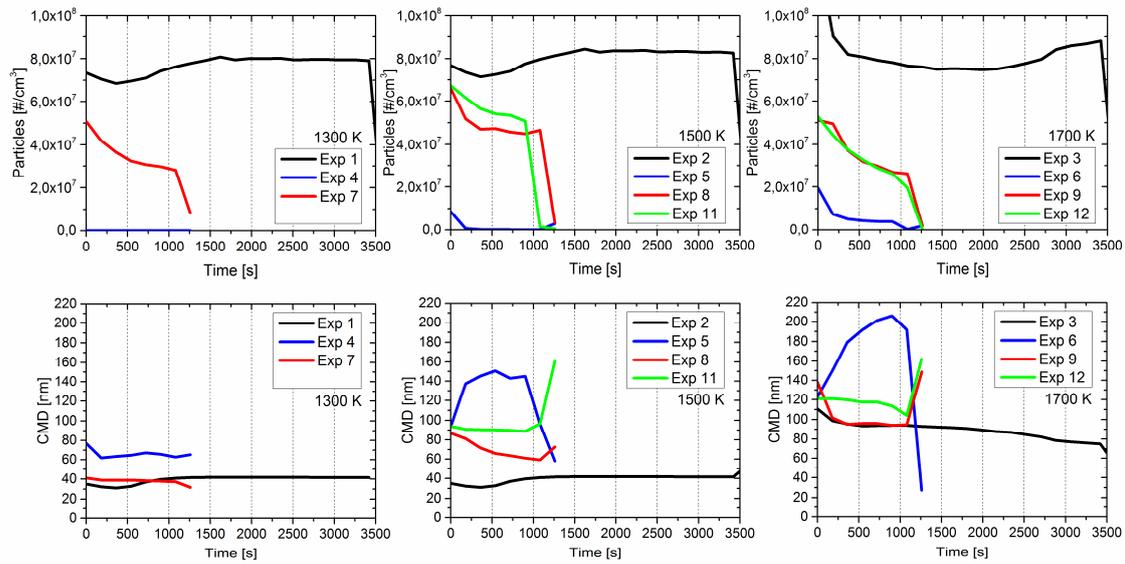
Figure 3. The particle number concentration [ $\#/cm^3$ ] (above) and count median diameter [nm] (below) at the outlet of the facility during experiments (measured with SMPS). The duration of experiments 1 to 3 was 60 minutes, whereas the rest of experiments lasted for 20 minutes.
