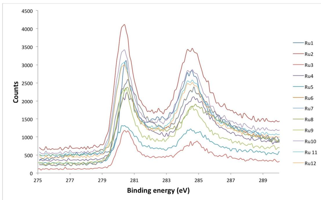
Figure 5. The obtained XPS spectra from the analysis of collected aerosols on filters.
