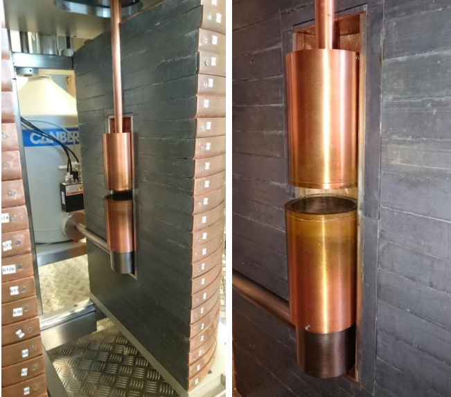
Figure 4. LGe system consisting of two planar Ge-detectors with epoxy window.
