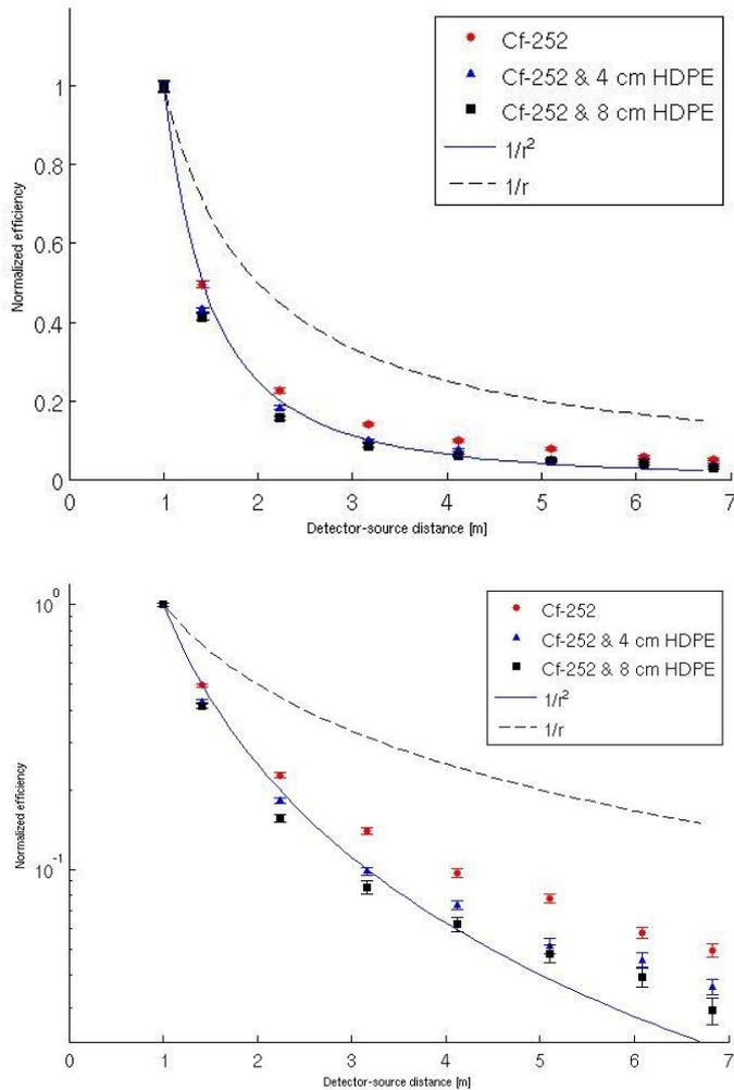
**Figure 3.** Normalized neutron count rate of the RanidPORT-N. The figure can be compared to figure 14.
