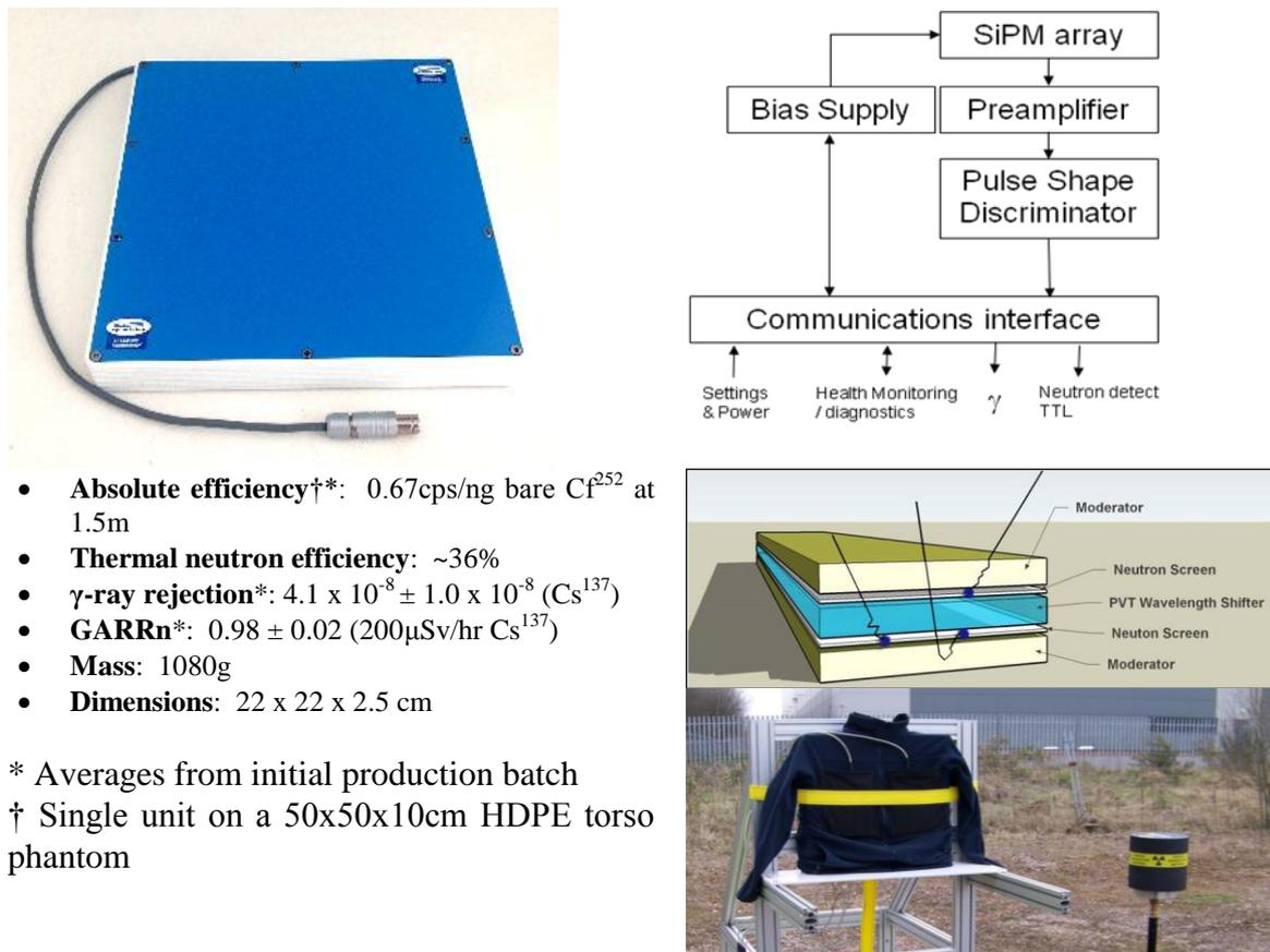
**Figure 11.** Clockwise: The instrument under test, its internal flow diagram, a single panel being tested for absolute efficiency, product specifications.
