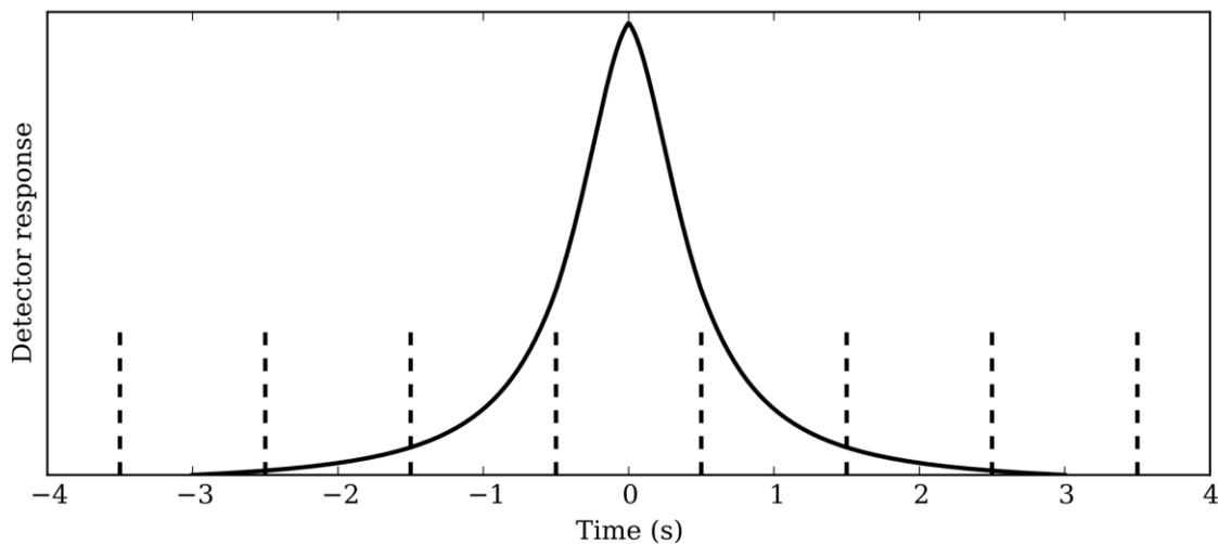
**Figure 4.** Theoretical response of a detector and a train of 1 second integrations.
