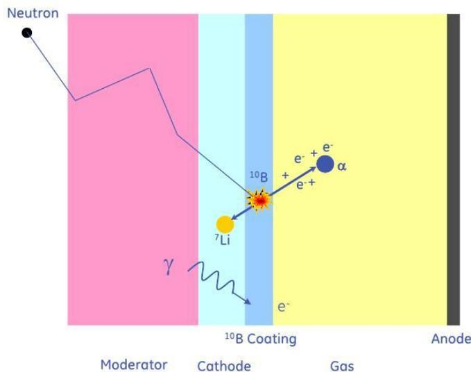
**Figure 7.**  $^{10}\text{B}$  neutron capture reaction in the boron layer of the detector.
