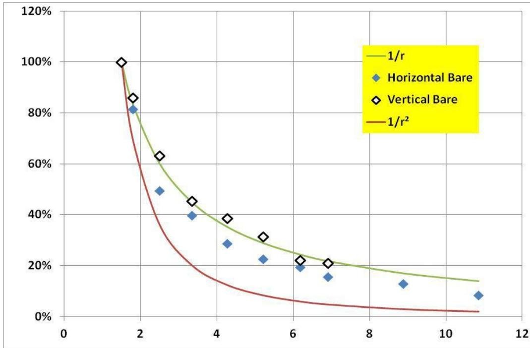
**Figure 14.** Normalized neutron count rate of the Thermo backpack. The x-axis shows the source-detector distance in meters.
