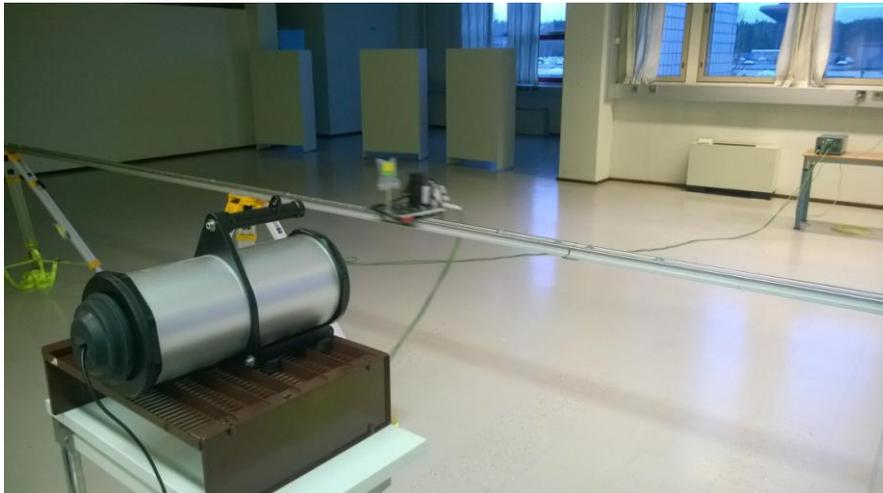
**Figure 1.** The testing track moving the source past STUKs BLASTER detector.
