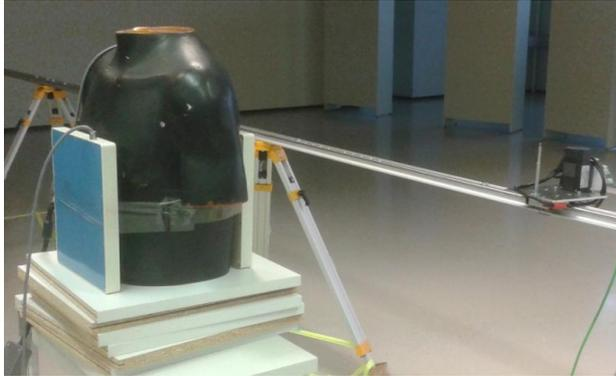
**Figure 12.** The test configuration for IEC 62694. The system is tested in ten orientations, rotated in two planes. Tests are carried out with both a bare and moderated (4cm HDPE)  $\text{Cf}^{252}$  source. Note that two units are fitted to the body phantom.
