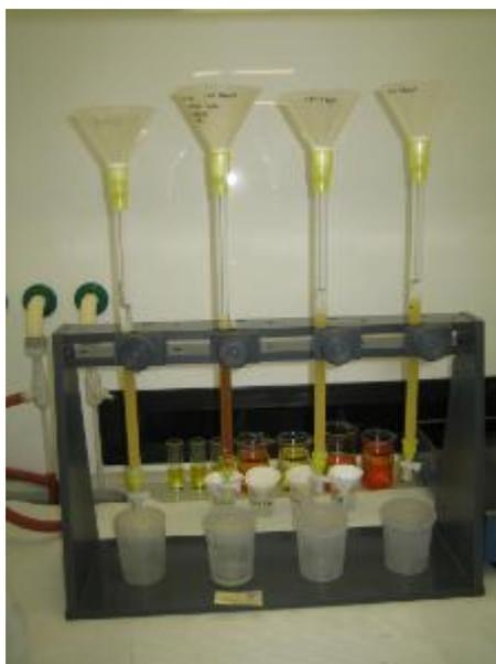
Figure. 11. Anion exchange columns
