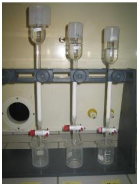
Figure. 10 Preconditioned Sr-resin columns ready to be used
