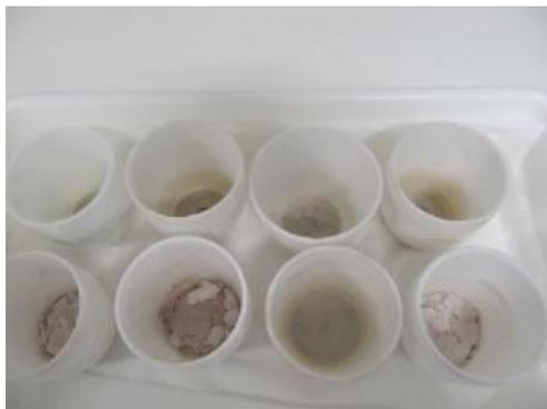
Figure. 9 Ashed oxalate precipitation in crucibles
