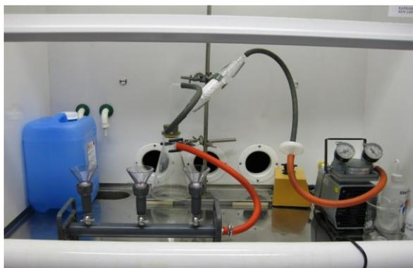
Figure. 21. Filtering apparatus for co-precipitated samples.
