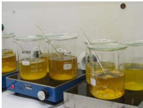
Figure. 7 Oxalate precipitation for soil sample
