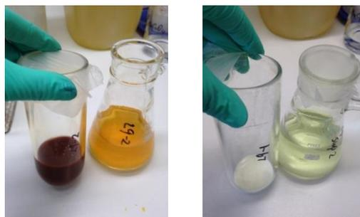
Figure. 17.  $\text{Fe}(\text{OH})_3$  precipitate (left) vs.  $\text{CaC}_2\text{O}_4$  precipitate (right) obtained after pre-concentration of 10 g Chinese soil
