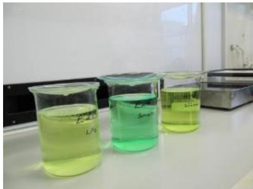
Figure. 8 Oxalate precipitation has settled (deposition sample)
