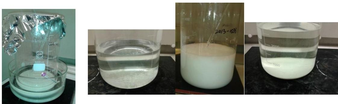
Figure. 15. Effect of temperature on the removal of Ca ( $\text{Ca}(\text{OH})_2$  treatment process in  $50^\circ\text{C}$  water bath (left 1) and following  $\text{SrCO}_3$  precipitation (left 2) vs.  $\text{Ca}(\text{OH})_2$  treatment process under room temperature (left 3) and the following  $\text{SrCO}_3$  precipitation (left 4)).
