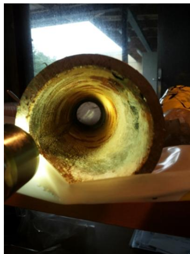
Figure 3. Visual appearance of the interior of a non-cleaned tube. The scale-thickness of the tube (tube No 7) was approximately 1mm.
