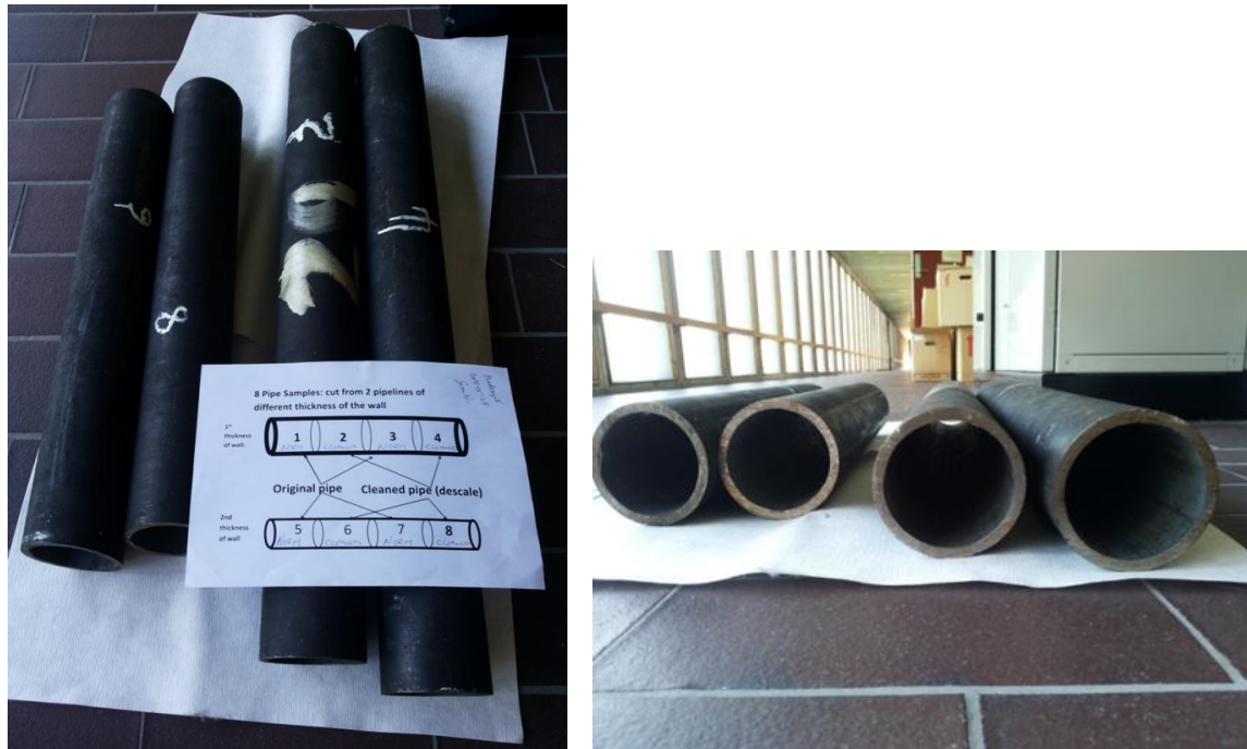
Figure 2. Steel pipes cleaned (descaled) from NORM by a decontamination company. The paper sheet shown on top of the tubes in the left picture shows the supposed cutting of the original tubes and the numbering of them, however later information revealed that the individual pipes were of different origin. Cleaned pipes were numbered No 2,4,6 and 8 while still contaminated pipes were No 1,3,5 and 7.
