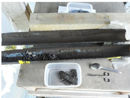
Figure 4. Tube cut along its axis with loose scale material inside.
