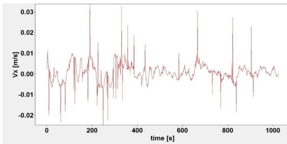
Figure 15. Velocity in x-direction in DCC-07-3 at the point 0,0 on the measurement plane.
