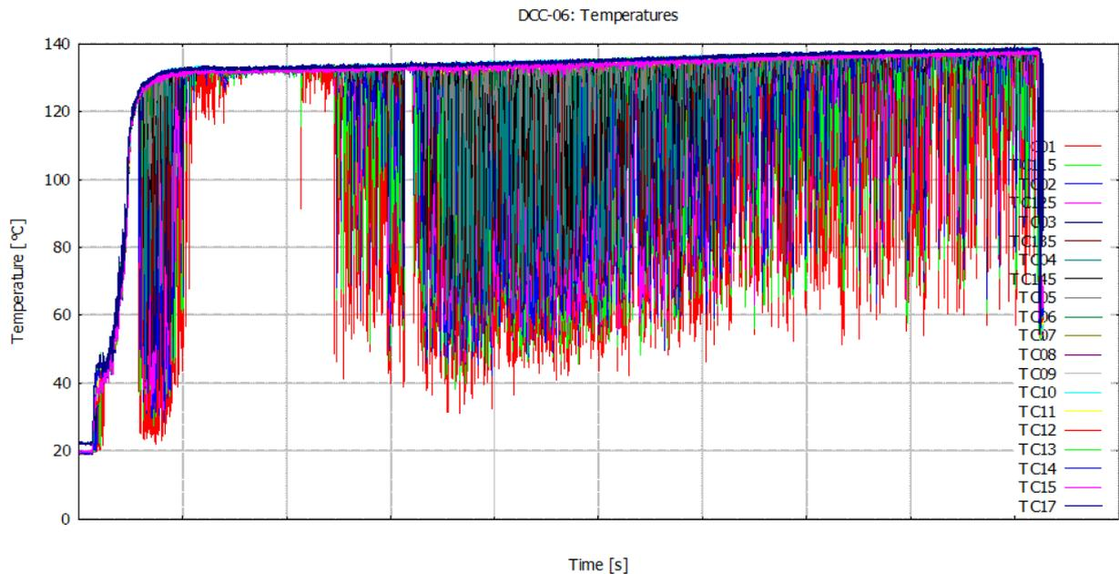
Figure 6. Temperature inside the blowdown pipe in the DCC-06 experiment.
