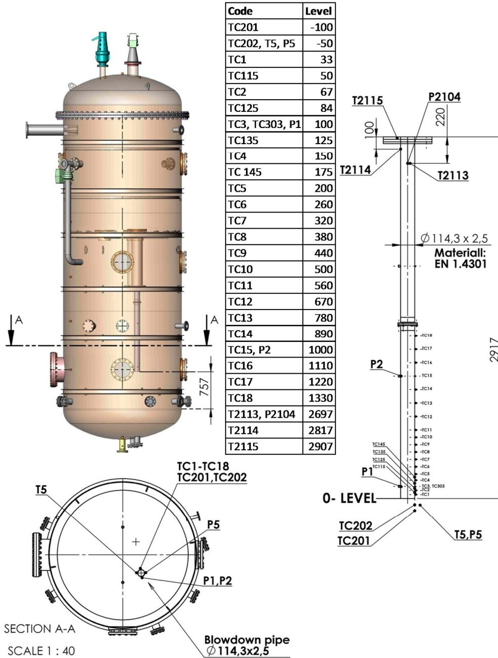
*Blowdown pipe measurements in the DCC-06 and DCC-07 tests.*
