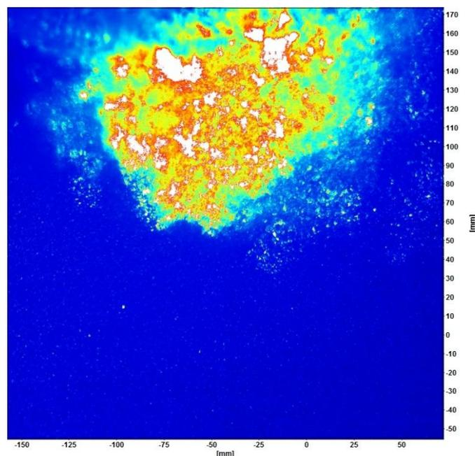
Figure 9. An example of oversaturated particle image caused by a huge steam release to the FOV.
