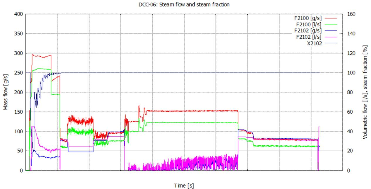
*Figure 4. Steam flow rate in the DCC-06 experiment.*
