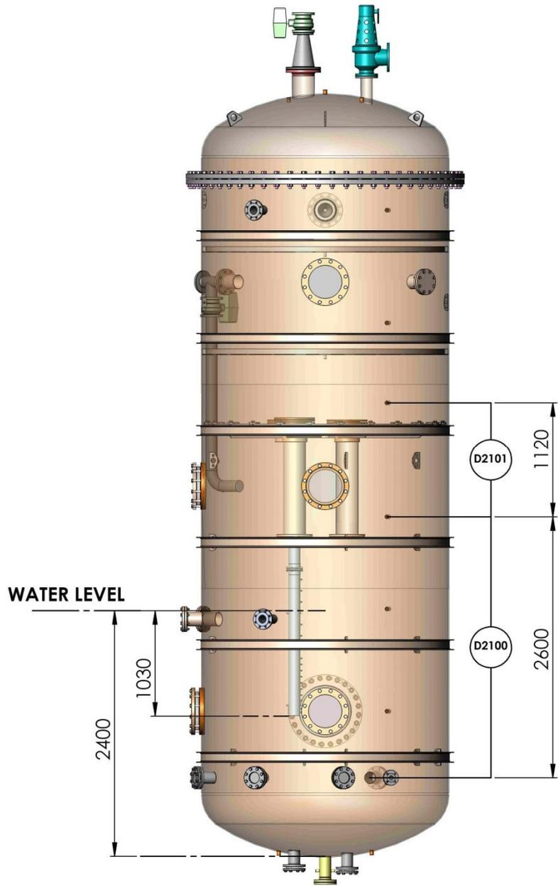
*Pressure difference measurements. Nominal water level is 2.4 m.*
