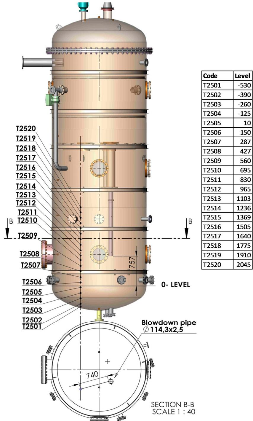
*Temperature measurements in the wetwell pool for the detection of thermal stratification.*
