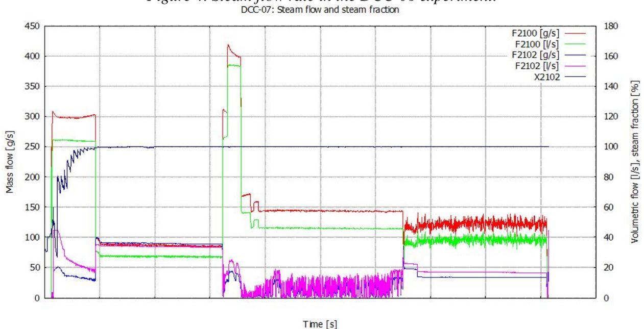
*Figure 5. Steam flow rate in the DCC-07 experiment.*
