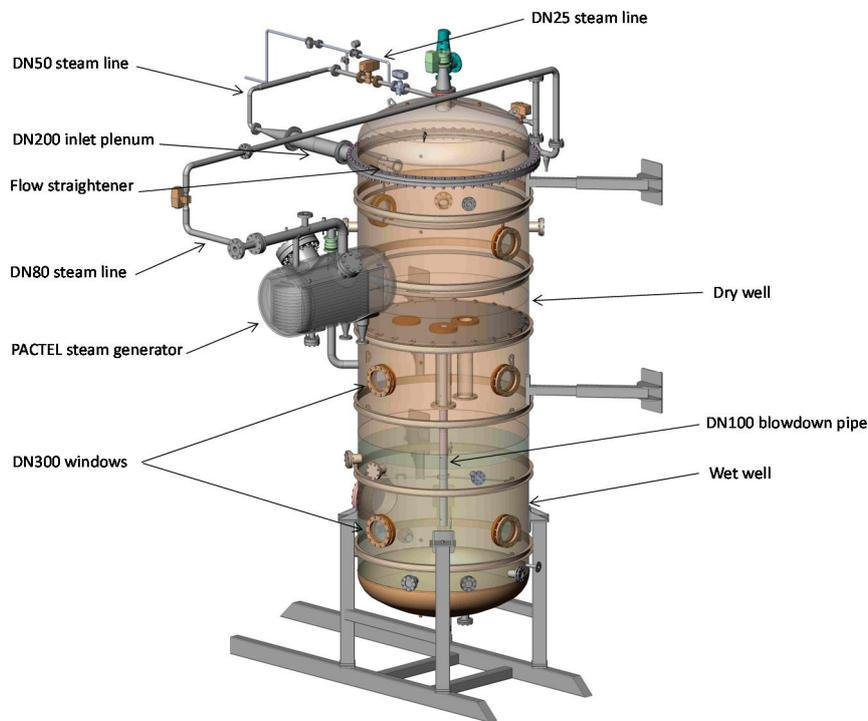
*Figure 2. PPOOLEX test vessel.*
