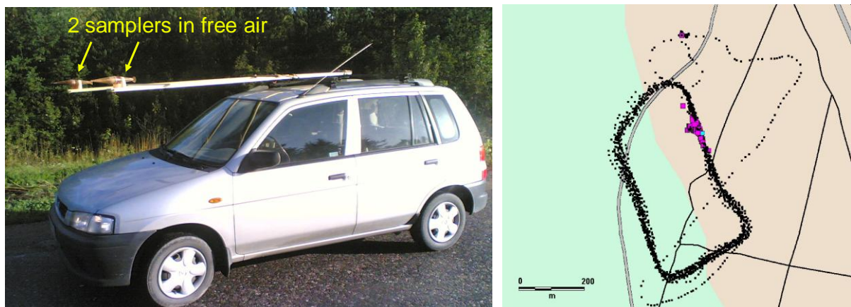
Figure 2. Testing operation of the MASS mini-UAV samplers using a car (left). Colored points in the right show the estimated location of the detected point source on the ground when the CsI detector is mounted in the mini-UAV. Black points refer to the route of the UAV during the flight test.
