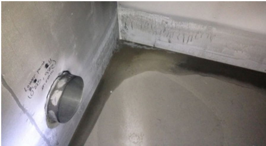
Figure 68 Close up picture of the connection pipe (200 mm) where the fan was connected. The picture is taken from inside the fire room; the fan was placed on the other side of the wall (outside).
