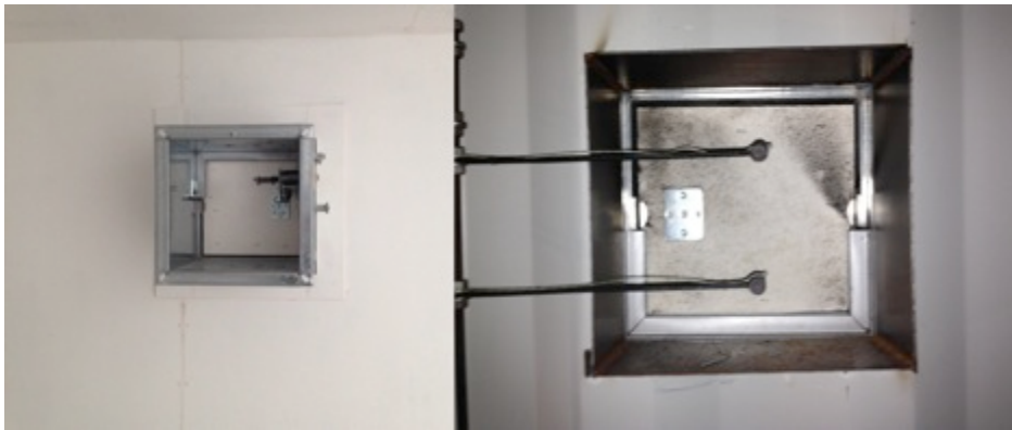
Figure 67 The placement of the fire damper, the left picture is from inside the fire room, the right picture is in the non-fire room where the bi-directional probes and coupled thermocouples were placed.
