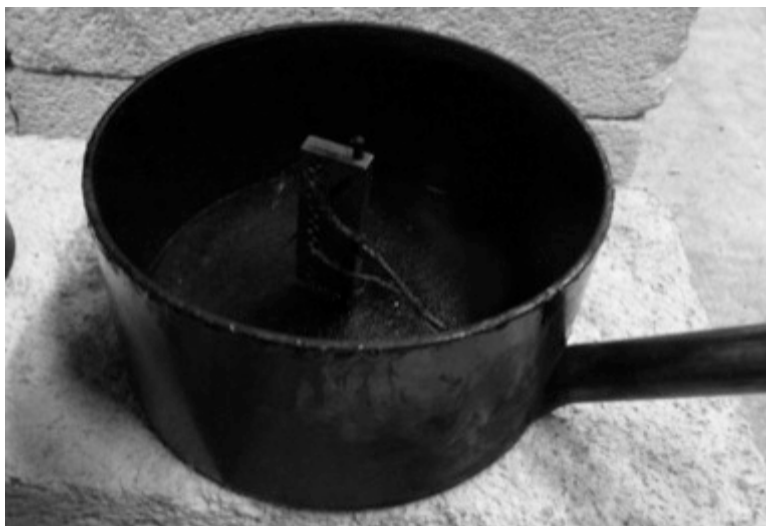
Figure 52 Thermocouples to measure liquid temperatures in the deep round cup sample holder
