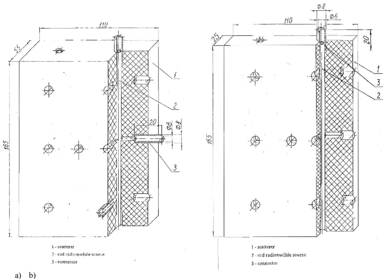
Figure 1. Module of scatter block with, a). One piece of radioactivity; b) Half piece of radioactivity.
