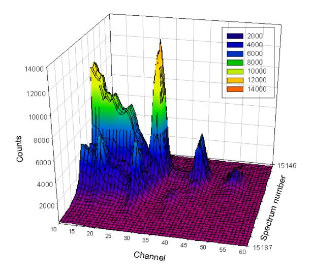
Figure 13. Graphical representation of the transition between Source 3 ( $^{192}$ Ir) and Source 4 ( $^{75}$ Se).
