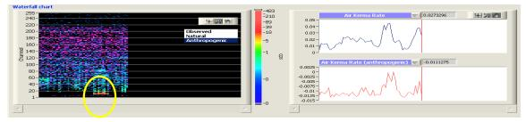
Source 9 (yellow) for the anthropogenic waterfall plot with automatic scaling. Source 8 is now not visible as an anthropogenic signal source due to the scaling from Source 9.
