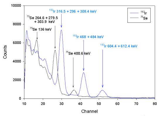
Figure 11. Comparison of summed spectra between 15146 to 15143 (solely <sup>192</sup>Ir) and 15172 to 15183 (solely <sup>75</sup>Se) showing similarities and differences.
