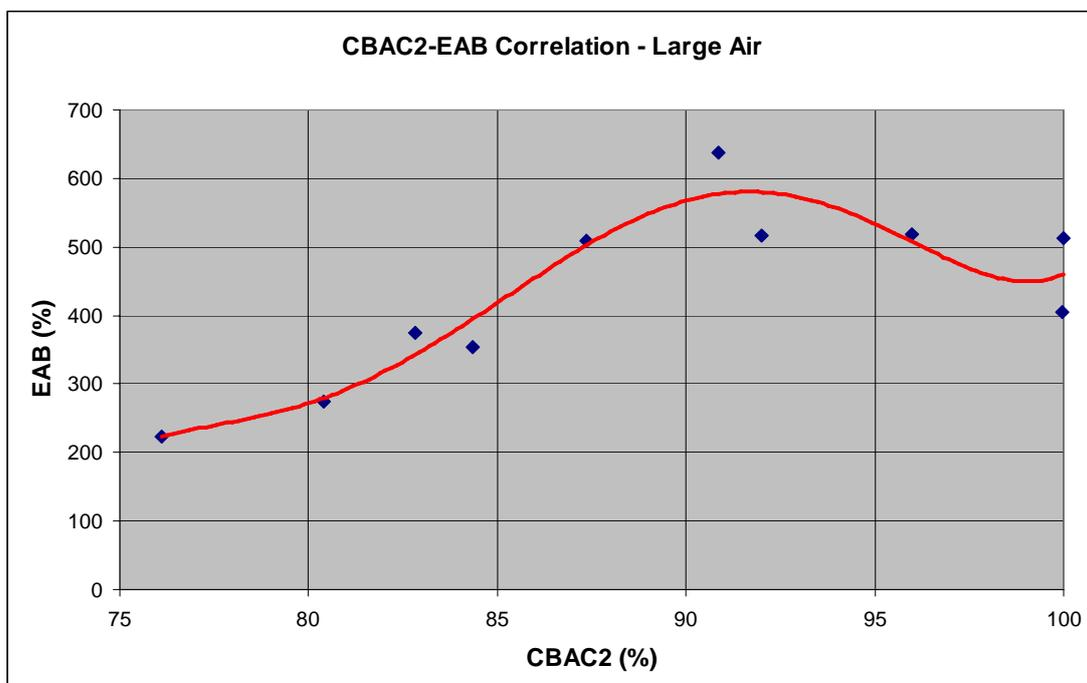
Figure 43 CBAC2/EAB correlation for the large type, air environment
