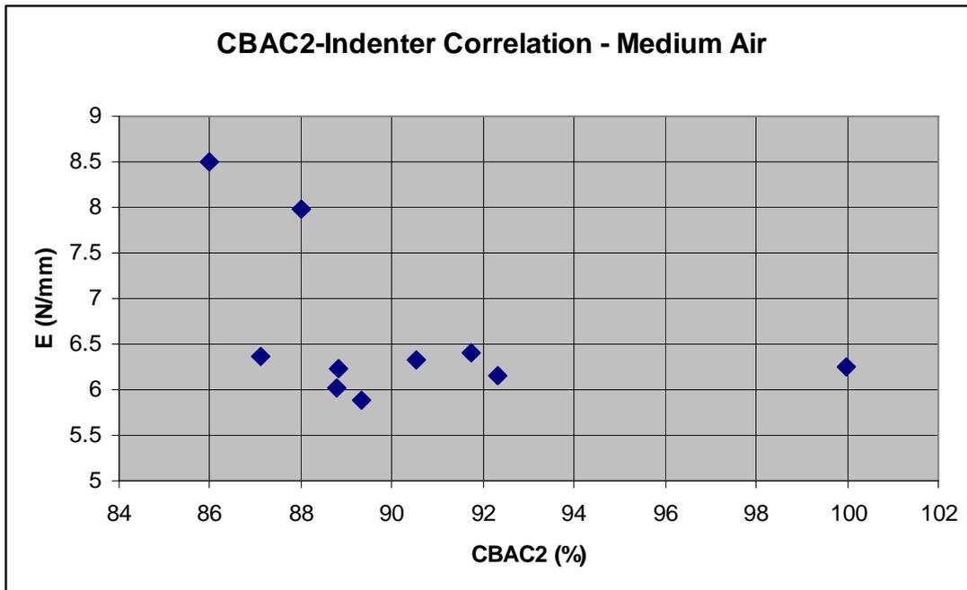
Figure 42 CBAC2/Indenter correlation for the medium type, air environment
