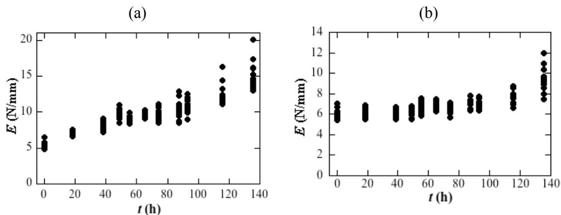
Figure 6. The indenter modulus as a function of ageing time for the jacketing (a) and the core insulation (b) for the large cable aged in air.
