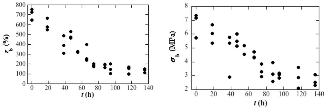
Figure 9. Tensile strain (a) and tensile stress (b) as functions of ageing times for core insulation from small cable aged in air.
