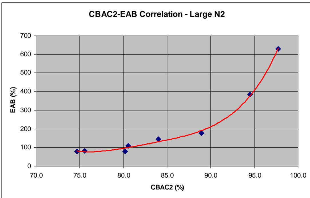
Figure 49 CBAC2/EAB correlation for the large type, N2 environment
