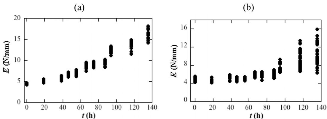
Figure 4. The indenter modulus as a function of ageing time for the jacketing (a) and the core insulation (b) for the small cable aged in air.
