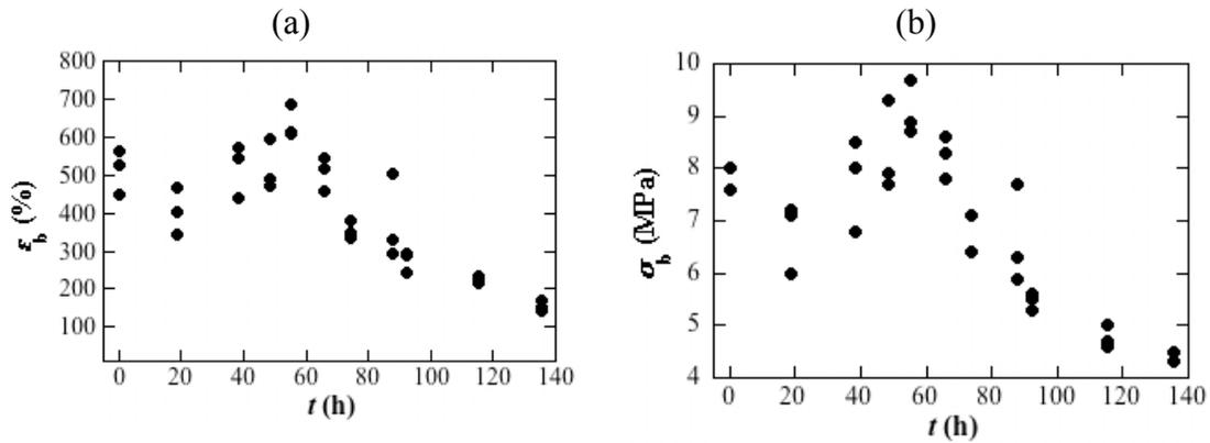
Figure 13. Tensile strain (a) and tensile stress (b) as functions of ageing times for core insulation from large cable aged in air.
