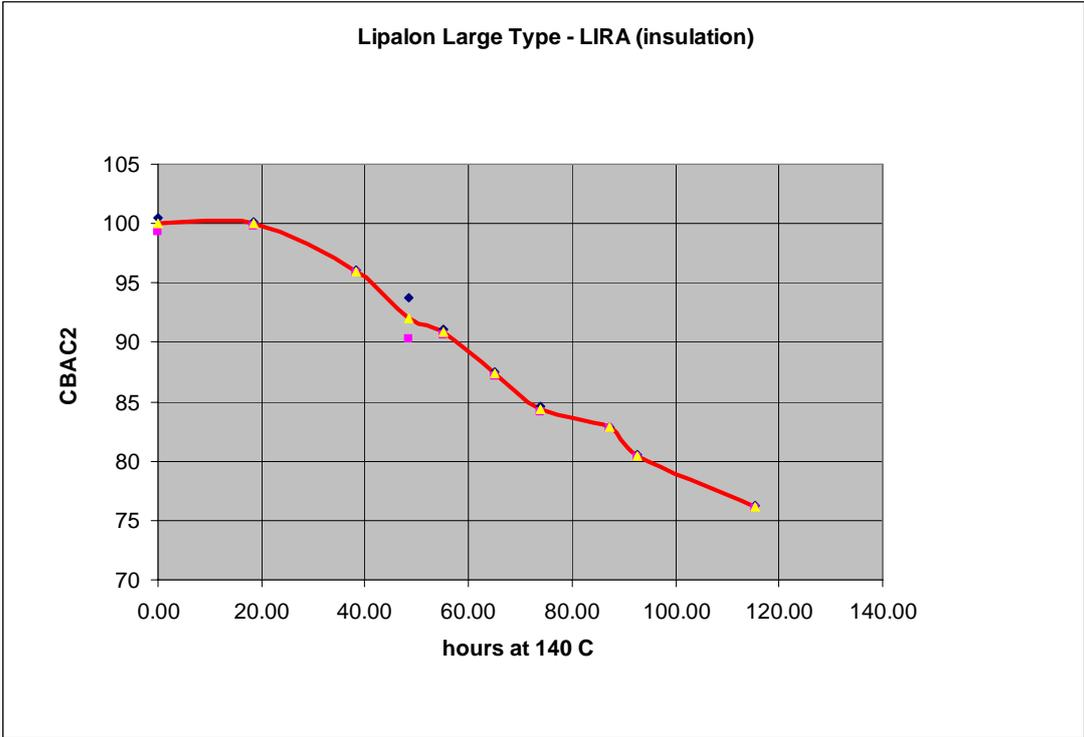
Figure 23 CBAC2 vs. ageing time, large type, air
