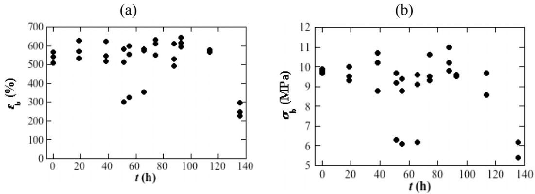
Figure 11. Tensile strain (a) and tensile stress (b) as functions of ageing times for core insulation from medium cable aged in air.
