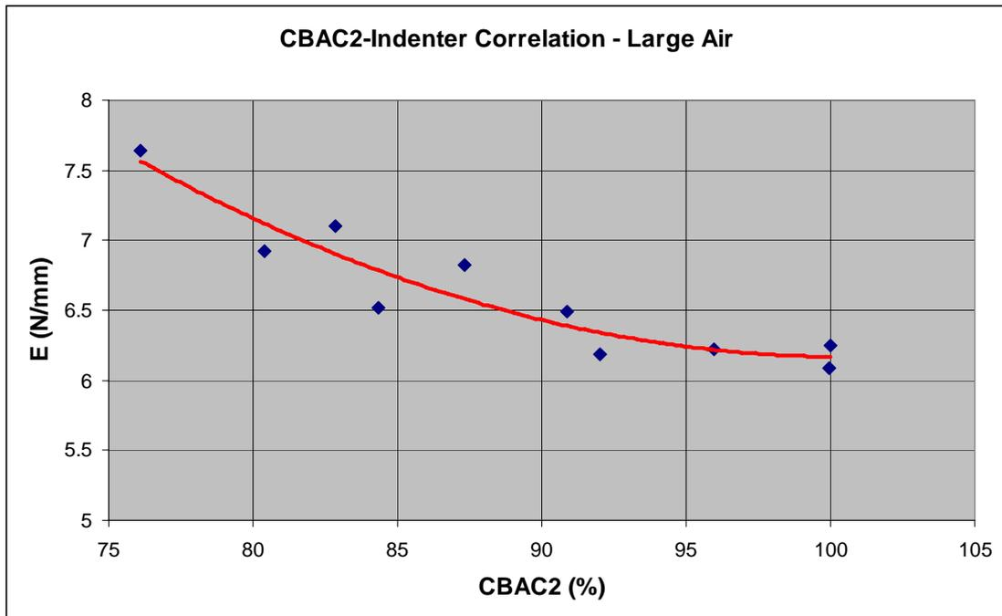
Figure 44 CBAC2/Indenter correlation for the largel type, air environment
