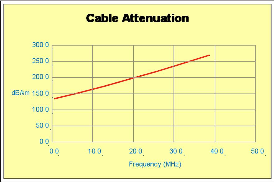
Figure 22 Attenuation spectrum, large type
