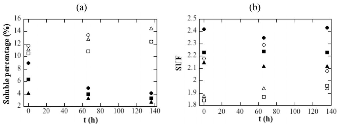
Figure 14. Soluble percentage (a) and solvent uptake factor (SUF) in (b) as functions of ageing time for small jacketing (●) and core insulation (○), medium jacketing (■) and core insulation (□) and large jacketing (▲) and core insulation (△)
