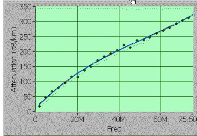
Figure 2 Cable attenuation (estimated by LIRA)
