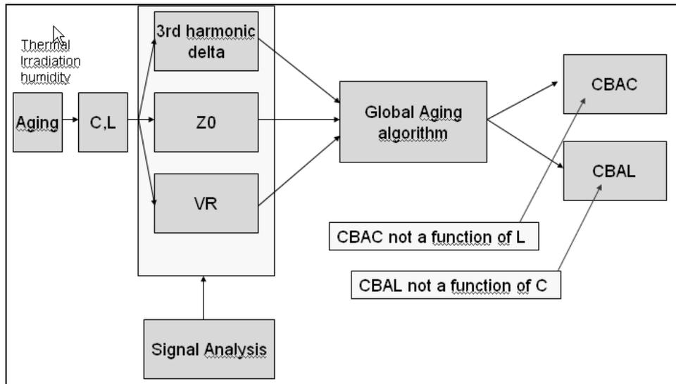
Figure 3 Global condition indicator algorithm
