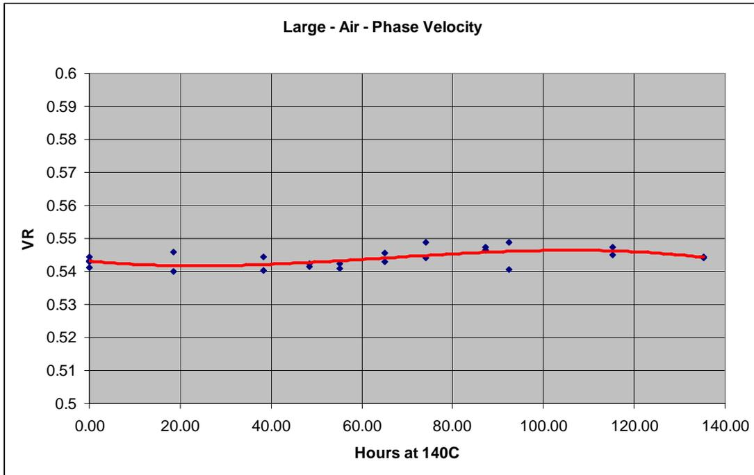
Figure 24 Velocity Ratio as a function of ageing time, medium air
