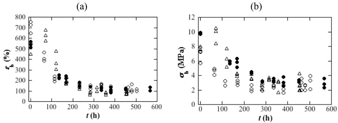
Figure 30. The tensile strain (a) and stress (b) as functions of ageing time for the jacketing the core insulation for the small (○), medium (●) and large (△) cable aged in nitrogen at 140°C.
