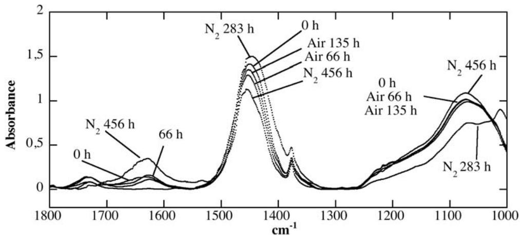
Figure 38. Spectra taken on samples aged in both air and nitrogen for the medium cable.
