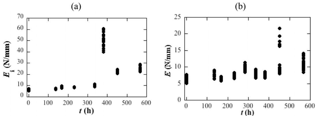
Figure 26. The indenter modulus as a function of ageing time for the jacketing (a) and the core insulation (b) for the medium cable aged in nitrogen at 140°C.
