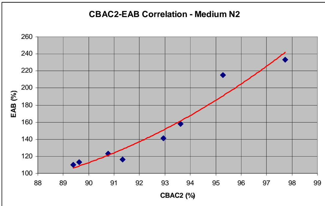
Figure 47 CBAC2/EAB correlation for the medium type, N2 environment
