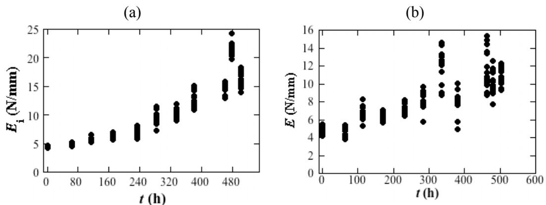
Figure 25. The indenter modulus as a function of ageing time for the jacketing (a) and the core insulation (b) for the small cable aged in nitrogen at 140°C.
