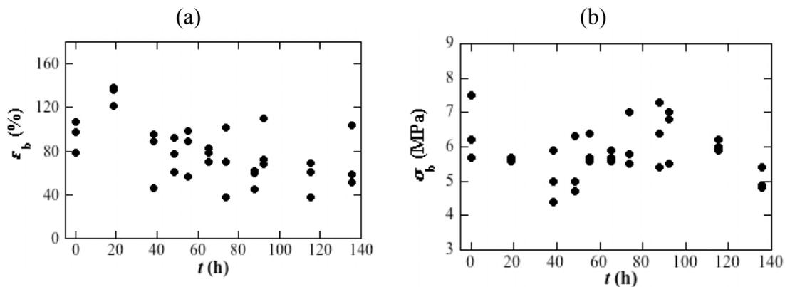
Figure 12. Tensile strain (a) and tensile stress (b) as functions of ageing time for jacketing from large cable aged in air.
