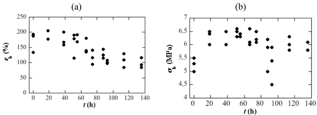
Figure 10. Tensile strain (a) and tensile stress (b) as functions of ageing times for jacketing from medium cable aged in air.
