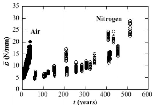
Figure 29. The data taken at 140°C are extrapolated to service temperatures at 50°C for all the three different cable samples aged in air and nitrogen.
