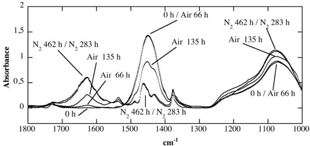
Figure 36. Spectra taken on samples aged in both air and nitrogen for the small cable.
