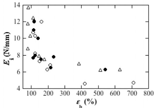
Figure 31. Indenter modulus,  $E_i$ , as a function of tensile strain,  $\epsilon_b$ , for the core insulation of the small (●), medium (▲) and large (○) cables aged in nitrogen.
