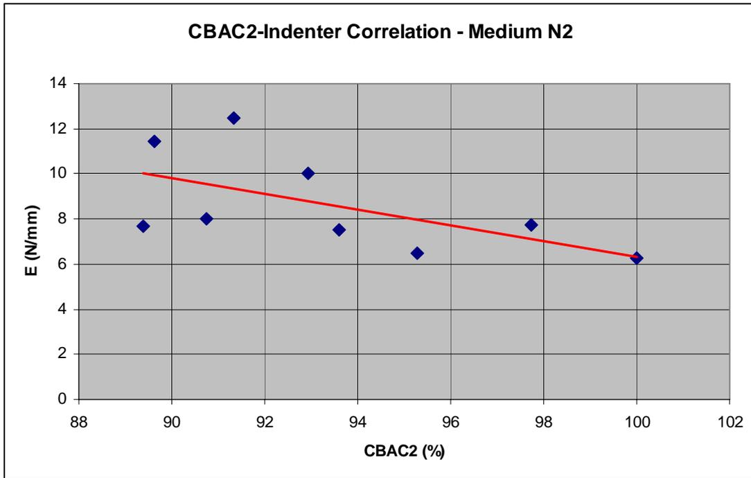
Figure 48 CBAC2/Indenter correlation for the medium type, N2 environment
