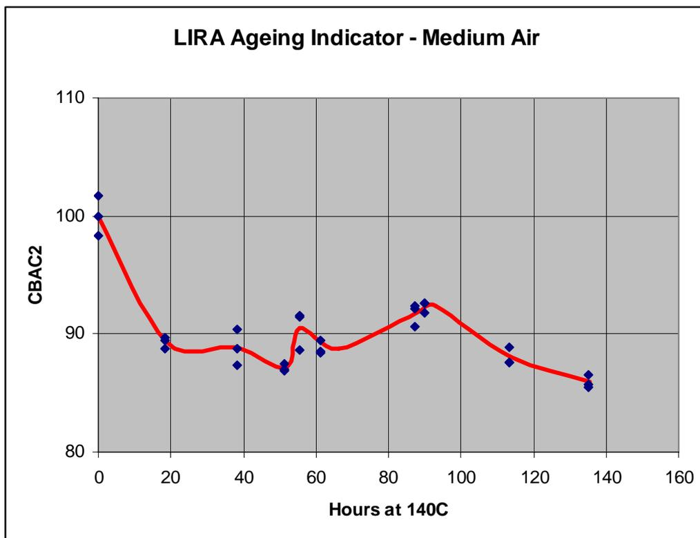
Figure 20 CBAC2 vs. ageing time, medium type, air
