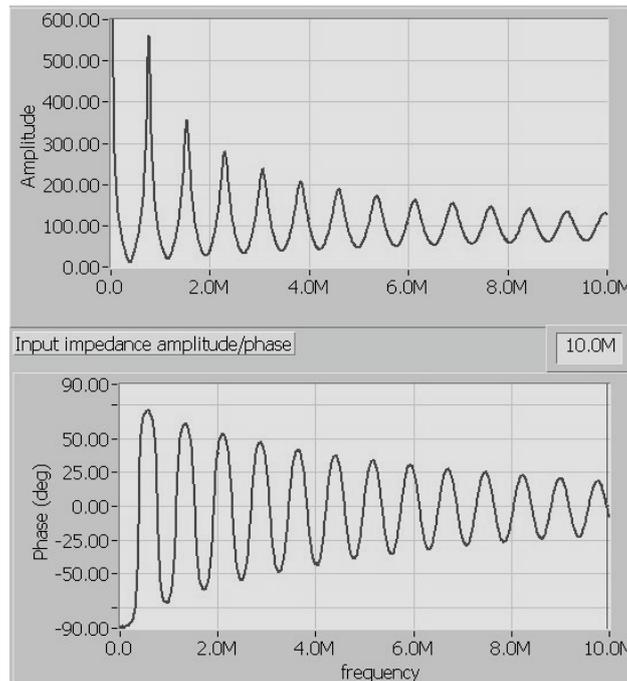
*Figure 1 Impedance spectrum of an unmatched transmission line.*
