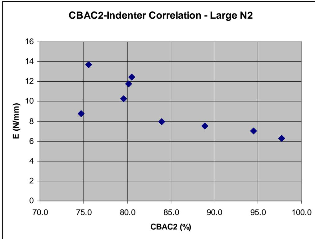
Figure 50 CBAC2/Indenter correlation for the large type, N2 environment
