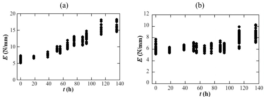
Figure 5. The indenter modulus as a function of ageing time for the jacketing (a) and the core insulation (b) for the medium cable aged in air.
