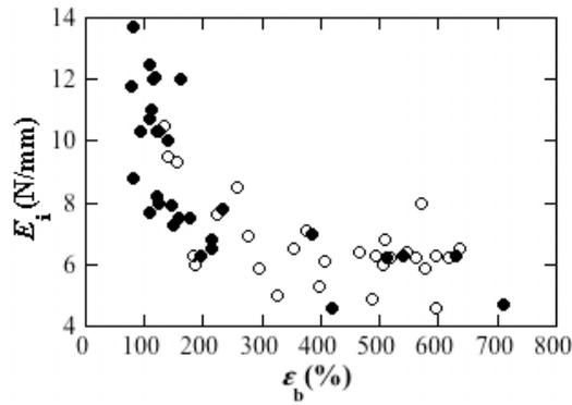
Figure 32. Indenter modulus,  $E_i$ , as a function of tensile strain,  $e_b$ , for the core insulation of all the cable samples aged in air (○) and in nitrogen (●).
