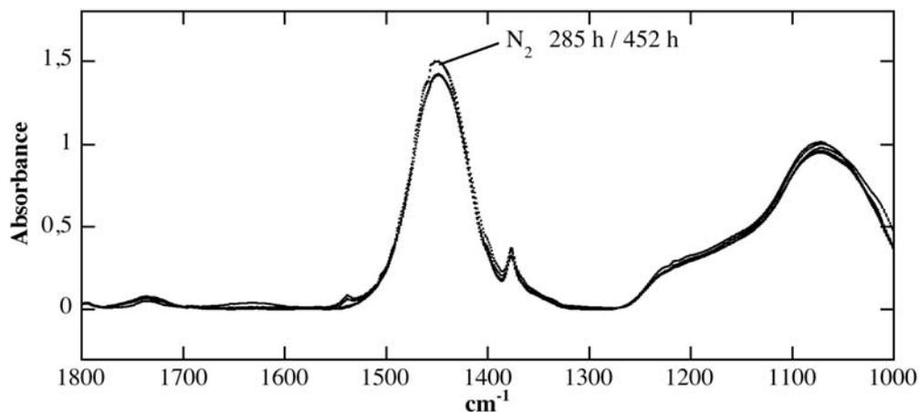
Figure 37. Spectra taken on samples aged in both air and nitrogen for the medium cable.
