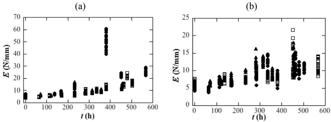
Figure 28. The indenter modulus as a function of ageing time for the jacketing (a) and the core insulation (b) for the small, medium and large cable aged in nitrogen at 140°C.
