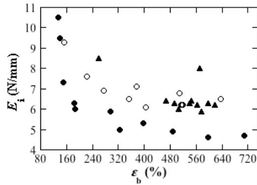
Figure 15. Indenter modulus,  $E_i$ , as a function of tensile strain,  $\epsilon_b$ , for the core insulation of the small (●), medium (▲) and large (○) cables.
