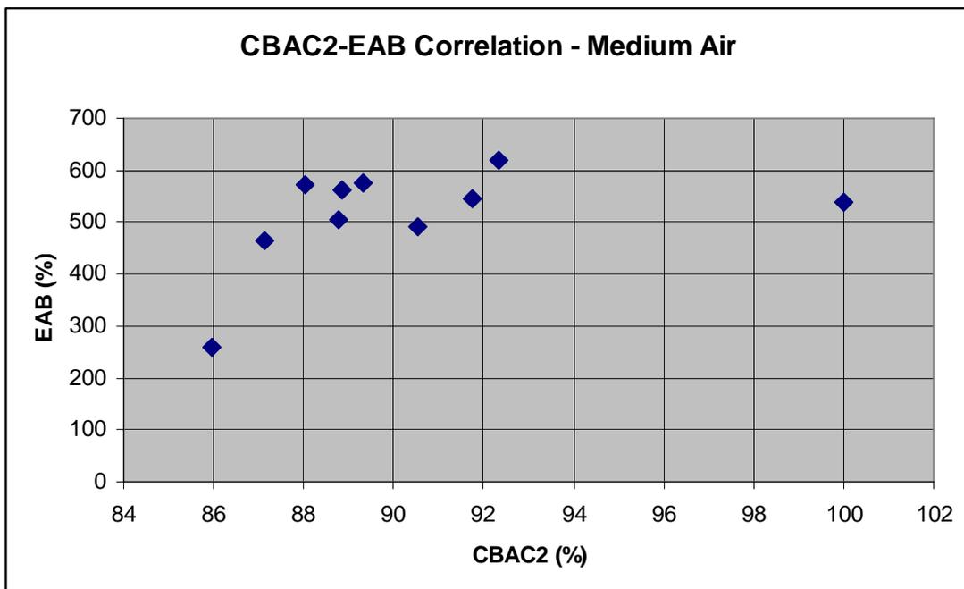
Figure 41 CBAC2/EAB correlation for the medium type, air environment
