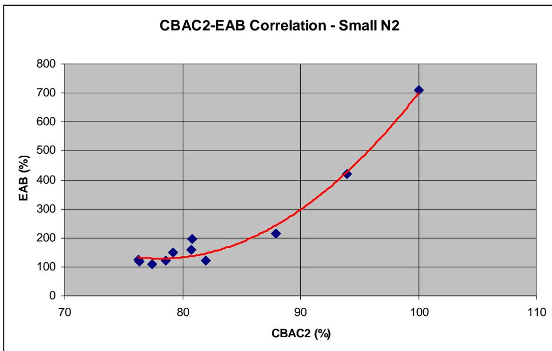
Figure 45 CBAC2/EAB correlation for the small type, N2 environment
