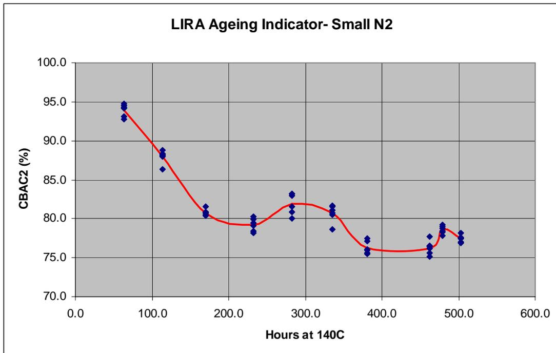
Figure 33 CBAC2 vs. ageing time, small type, N2
