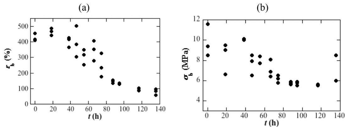
Figure 8. Tensile strain (a) and tensile stress (b) as functions of ageing times for jacketing from small cable aged in air.
