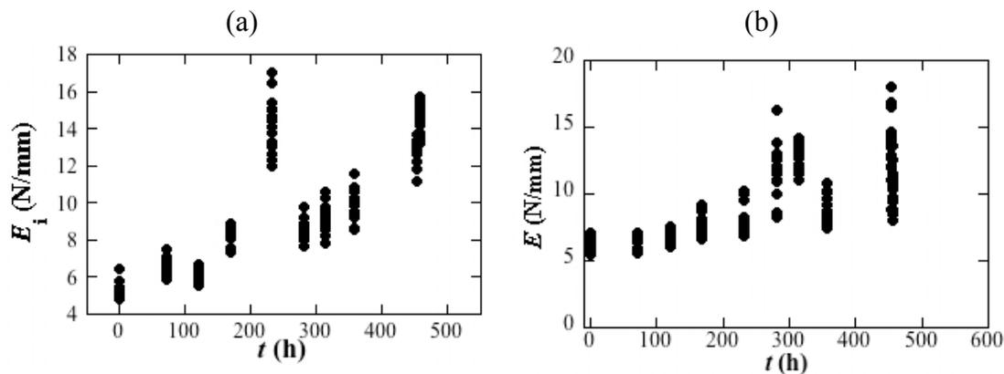
Figure 27. The indenter modulus as a function of ageing time for the jacketing (a) and the core insulation (b) for the large cable aged in nitrogen at 140°C.
