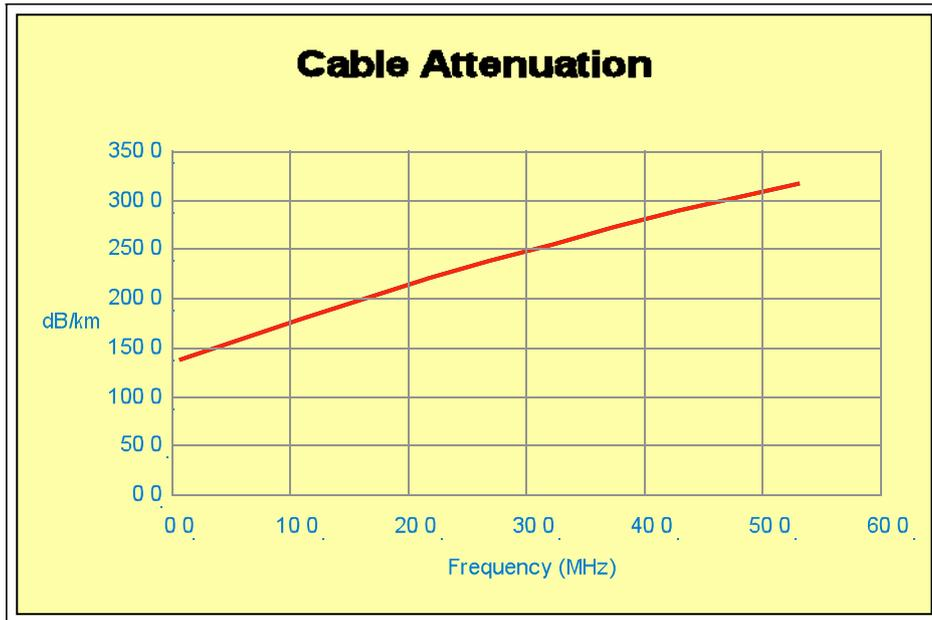
Figure 19b Attenuation spectrum, medium type
