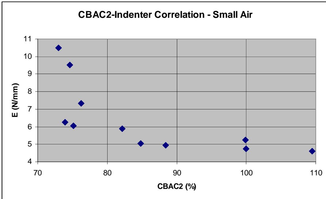
Figure 40 CBAC2/Indenter correlation for the small type, air environment
