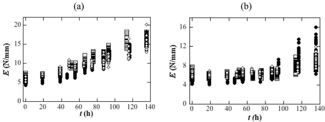
Figure 7. The indenter modulus as a function of ageing time for the jacketing (a) and core insulation (b) for small cable (●), medium cable (□) and large cable (◇).
