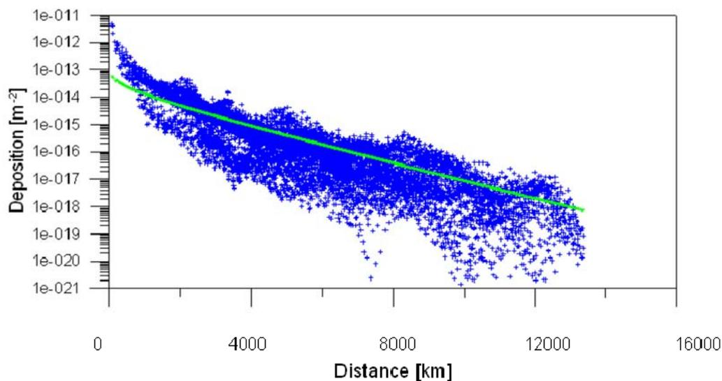
Figure 4. Annual mean deposition of  $^{137}\text{Cs}$  as function of the distance from the release site (Leningrad NPP, 1983 data). The average (inserted curve) results from a non-linear regression to the deposition data.
