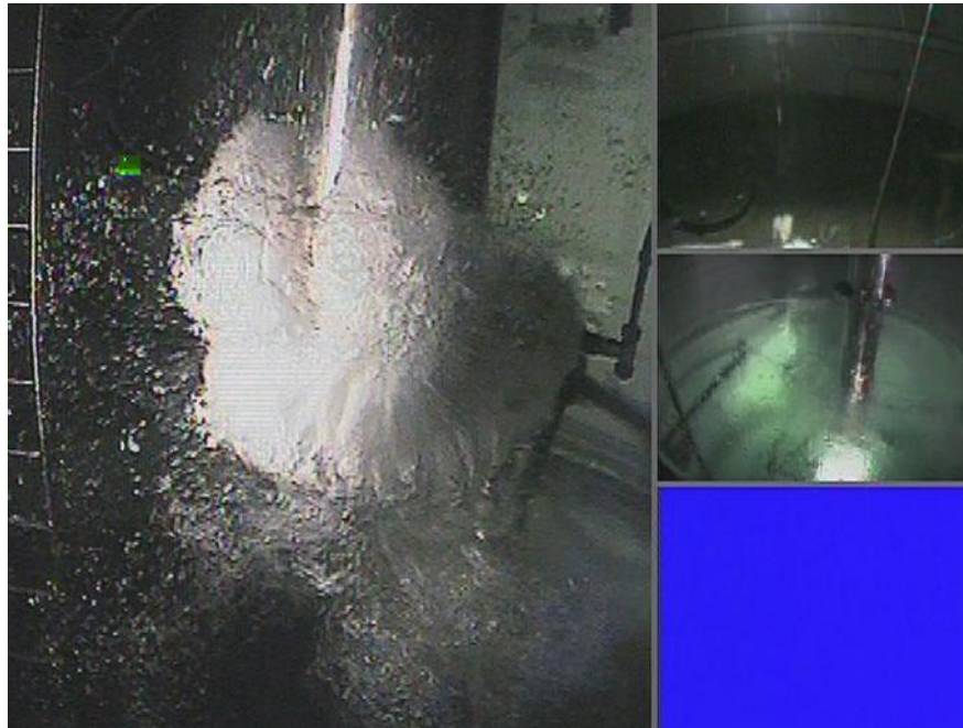
Figure 4. Typical camera views from the STR experiments in 2010 (STR-09, chugging condensation mode).
