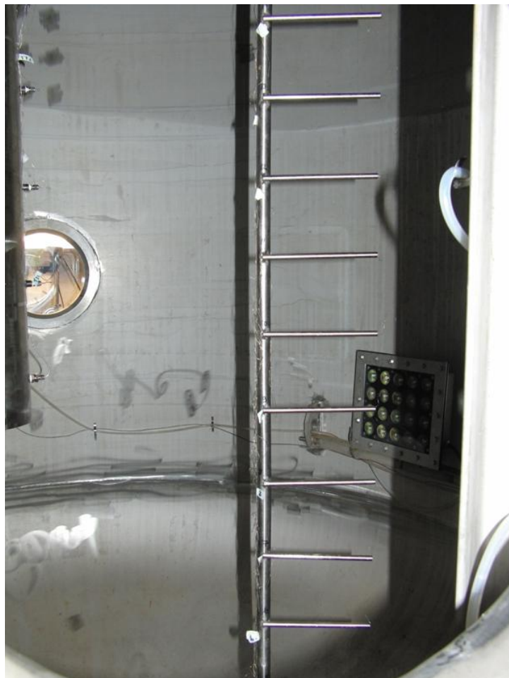
Thermocouples(T501...T516) for measuring vertical temperature distribution.
