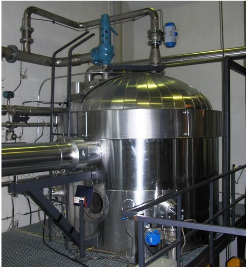
Thermally insulated dry well compartment and inlet plenum.
