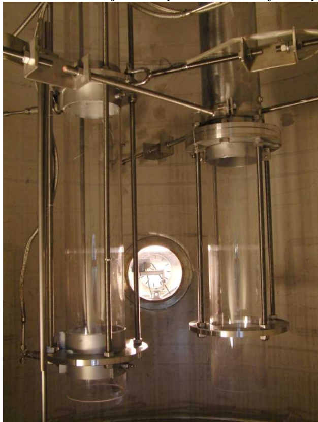
Lower parts of the blowdown pipes. Pipe 1 is on the left and pipe 2 on the right.
