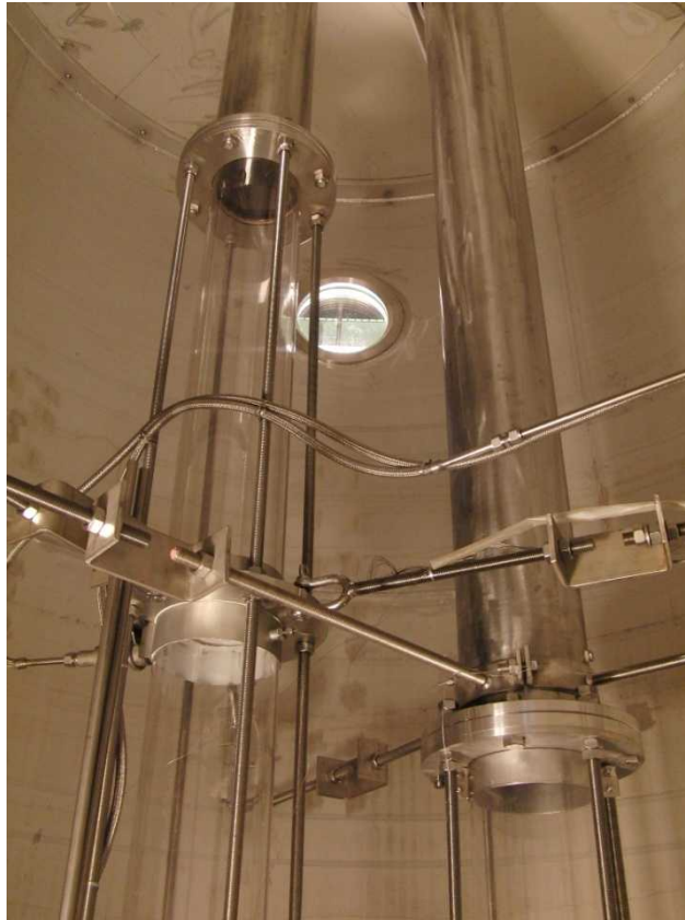
Blowdown pipes and intermediate floor. Pipe 1 is on the left and pipe 2 on the right.
