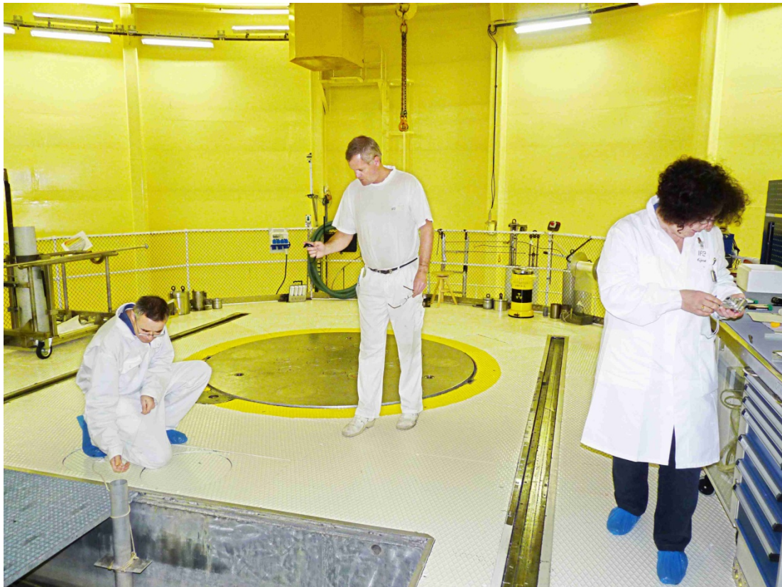
Figure 3. A photograph of the IFE exposure facility. Andrzej Wojcik (left) is kneeling and holding a blood tube inside the aluminium tube. Alicja Jaworska (right) is preparing the next sample for exposure. John Arild Tellevik (middle) is taking the time with a stopwatch.
