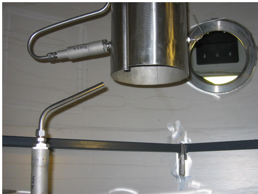
Pressure and temperature measurements at the blowdown pipe outlet.
