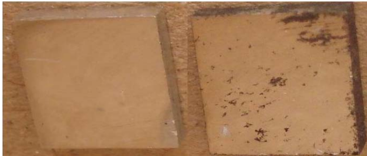
a) Aluminium, before and after RuO 4 treatment
