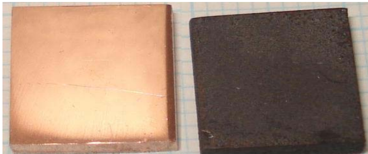
b) Copper, before and after RuO 4 treatment
