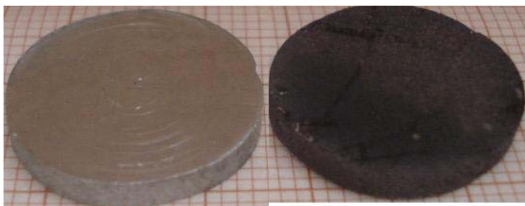
c) Zinc, before and after RuO 4 treatment
