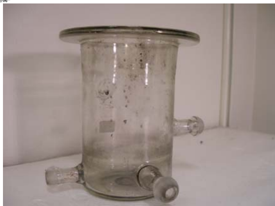
Figure 3.1: The reaction vessel after the completed experiments. Observe the black spots of ruthenium deposits.
