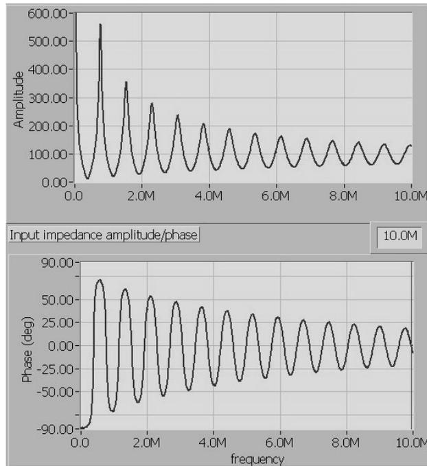
*Figure 1. Impedance of an unmatched transmission line.*
