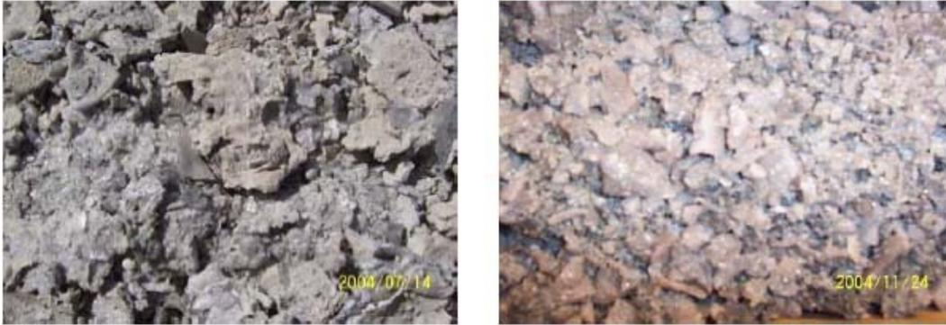
Figure 9. Structure of debris upper layer from COMECO top-flooding tests.
