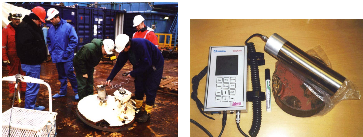
Figure 2. Left: Dose rate measurements at Regalia, of a piece of the inner hull from Kursk. Right: A NaI spectrum from a piece of the inner hull of Kursk (compartment VIII) is obtained.
