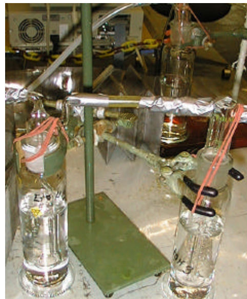
Figure 7. Iodine traps, NaOH and ethanol in bubblers.
