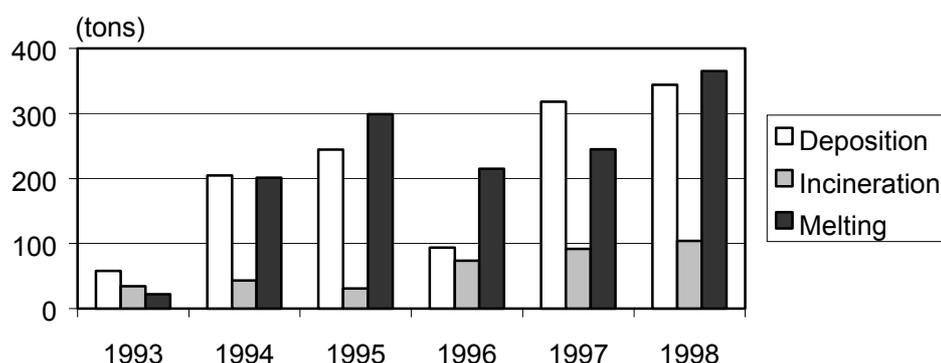
**Figure 1.** Diagram. Amount of material released from regulatory control by deposition, incineration of oil or melting of metals during 1993-1998.
