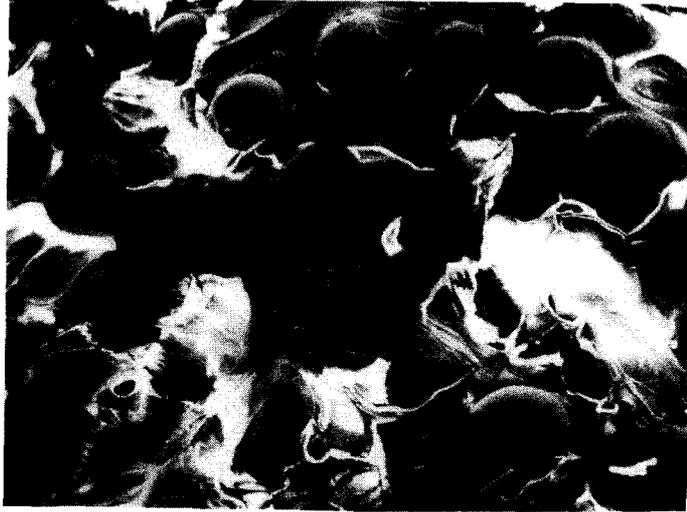
Figure 5-4. Mixed bed bead resin to bitumen ratio = 50:50 w%. Stored dry in a refrigerator for ca 4 years. Water content 4.9%. SEM 35x. The pictures show the preferential orientation of the cracks from bead to bead. Also the diameter of the relatively dry beads can be measured fairly accurately.
