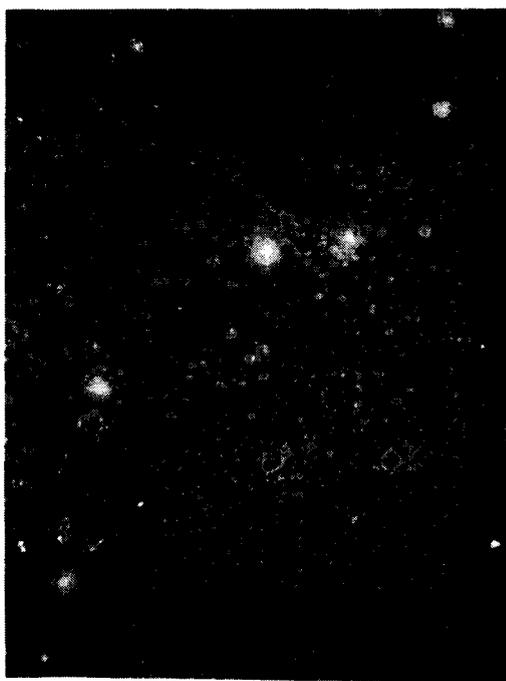
Figure 7-9. Colonies of micro-organisms on the surface of pure Mexphalte 40/50 four months after inoculation. The sample was kept under aerobic conditions in a nutrient solution /28/.
