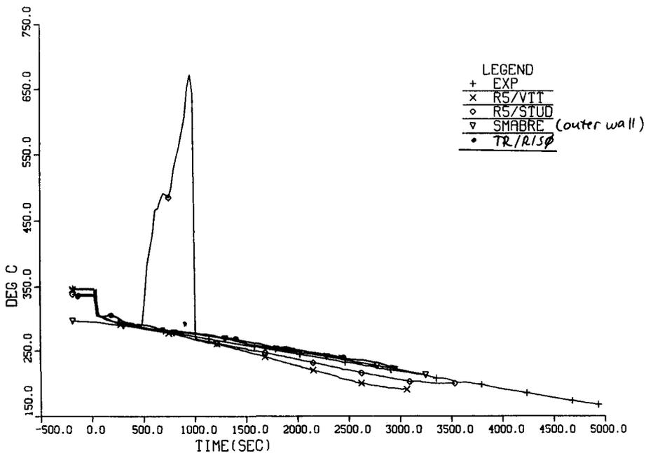
Figure 3.4.8 Rod temperature in middle core region (level 7).
