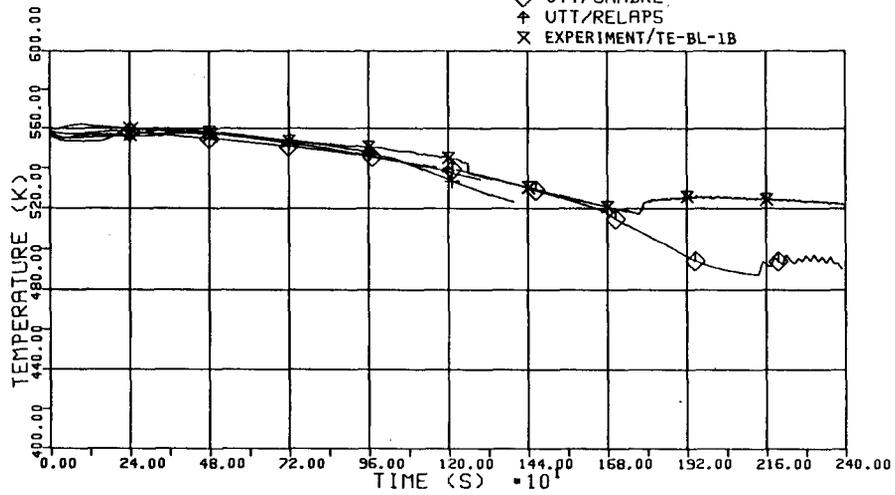
Fig. 3.1.3.2 Temperature in broken loop cold leg
