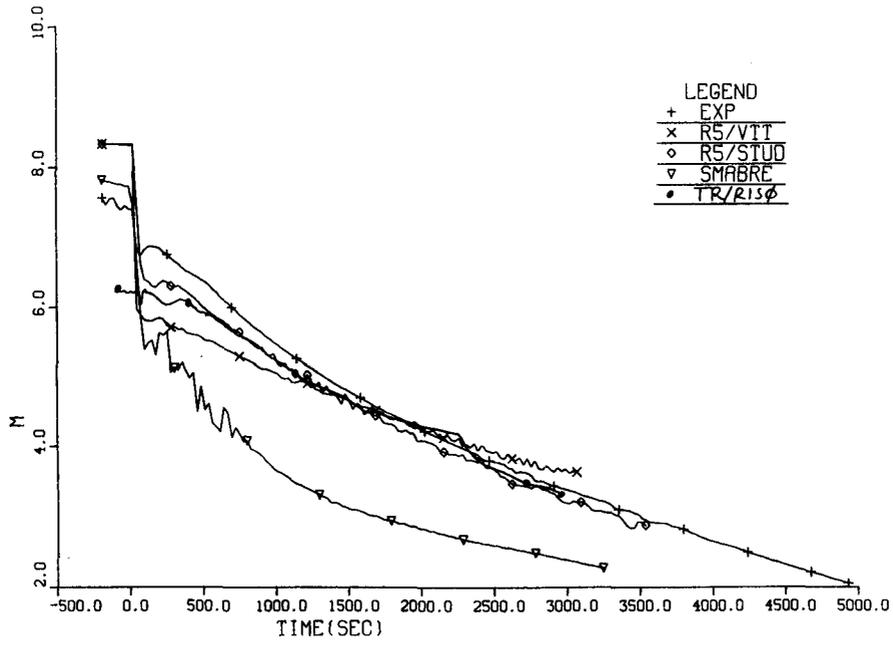
Figure 3.4.10 Collapsed liquid level in downcomer of intact loop steam generator.
