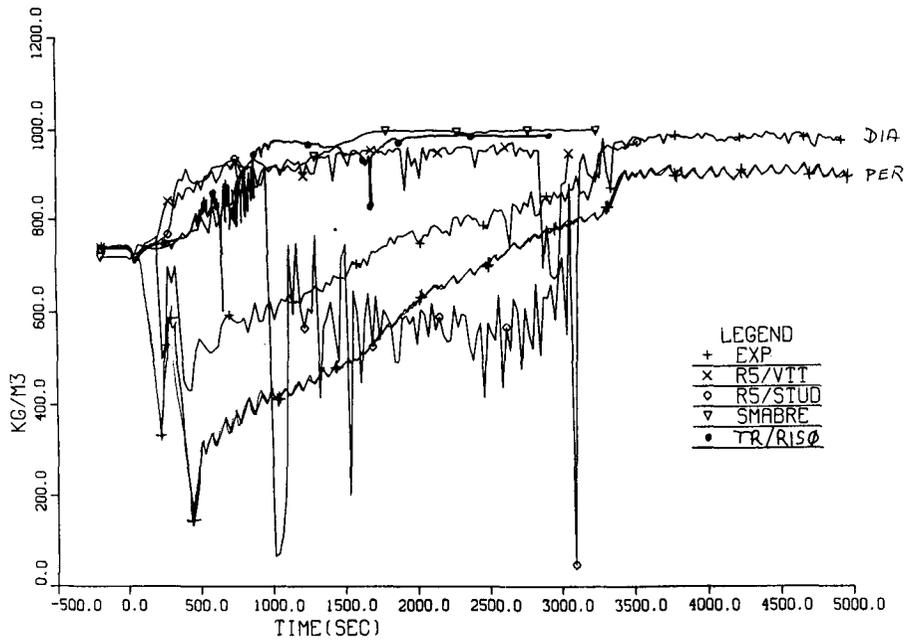
Figure 3.4.5 Mixture density in intact loop cold leg (vessel inlet).
