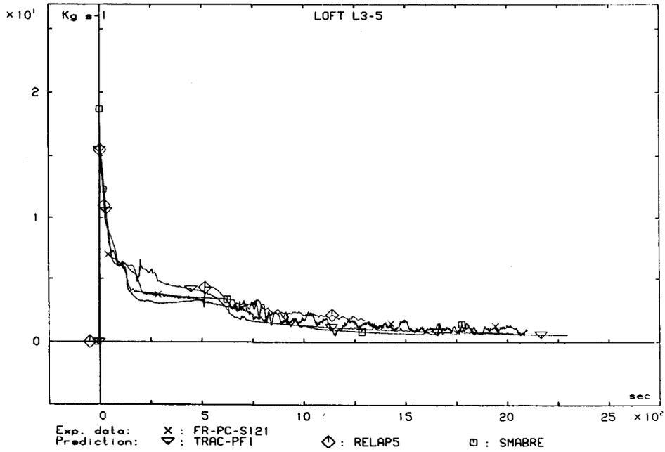
Fig. 3.1.4.6 Break mass flow
