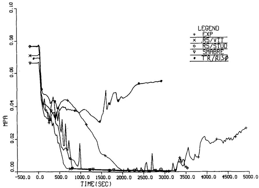
Figure 3.4.7 Differential pressure over broken loop steam generator ascending U-tube leg.
