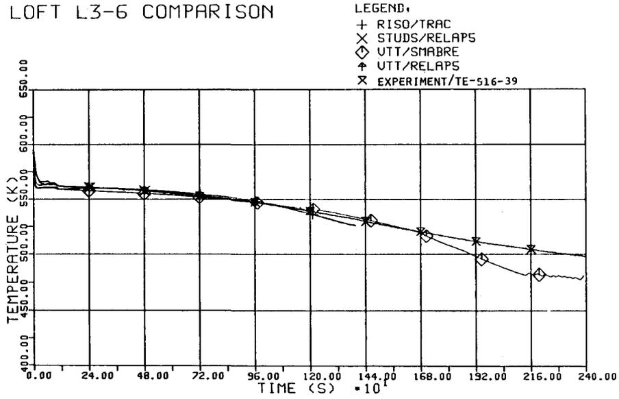
Fig. 3.1.3.3 Cladding temperature, average rod at 39 inch elevation
