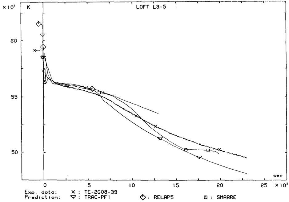
Fig. 3.1.4.3 Cladding temperature, average rod at 39 inch elevation
