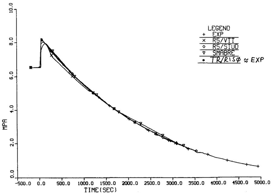
Figure 3.4.9 Secondary pressure in steam dome of intact loop steam generator.
