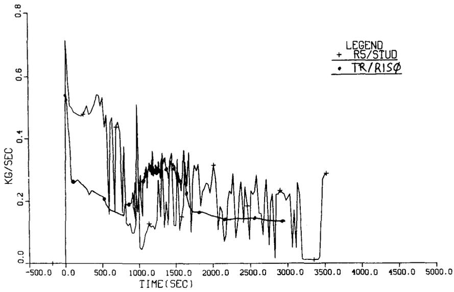
Figure 3.4.1 Break mass flow rate.
