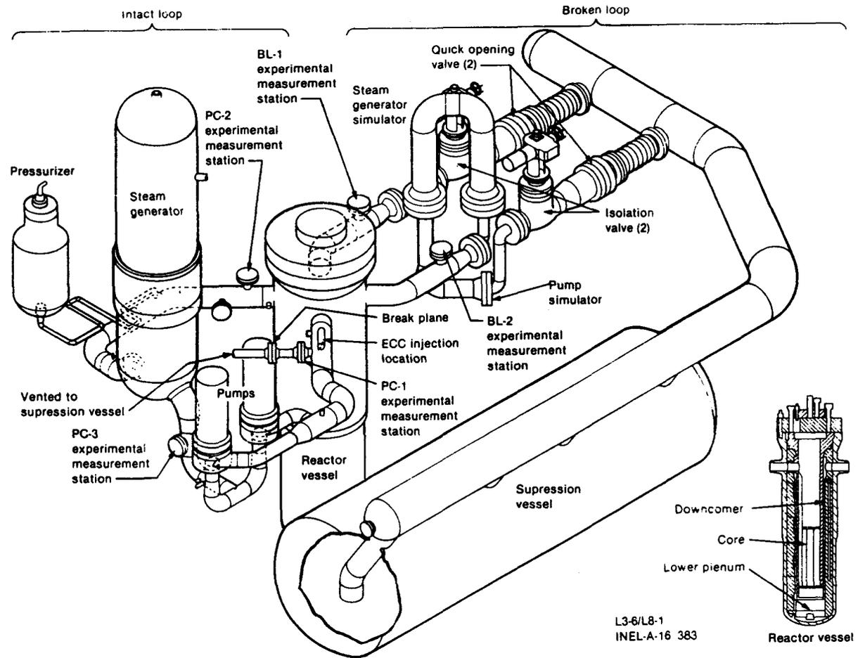
Figure A.1. Axonometric projection of LOFT system.
