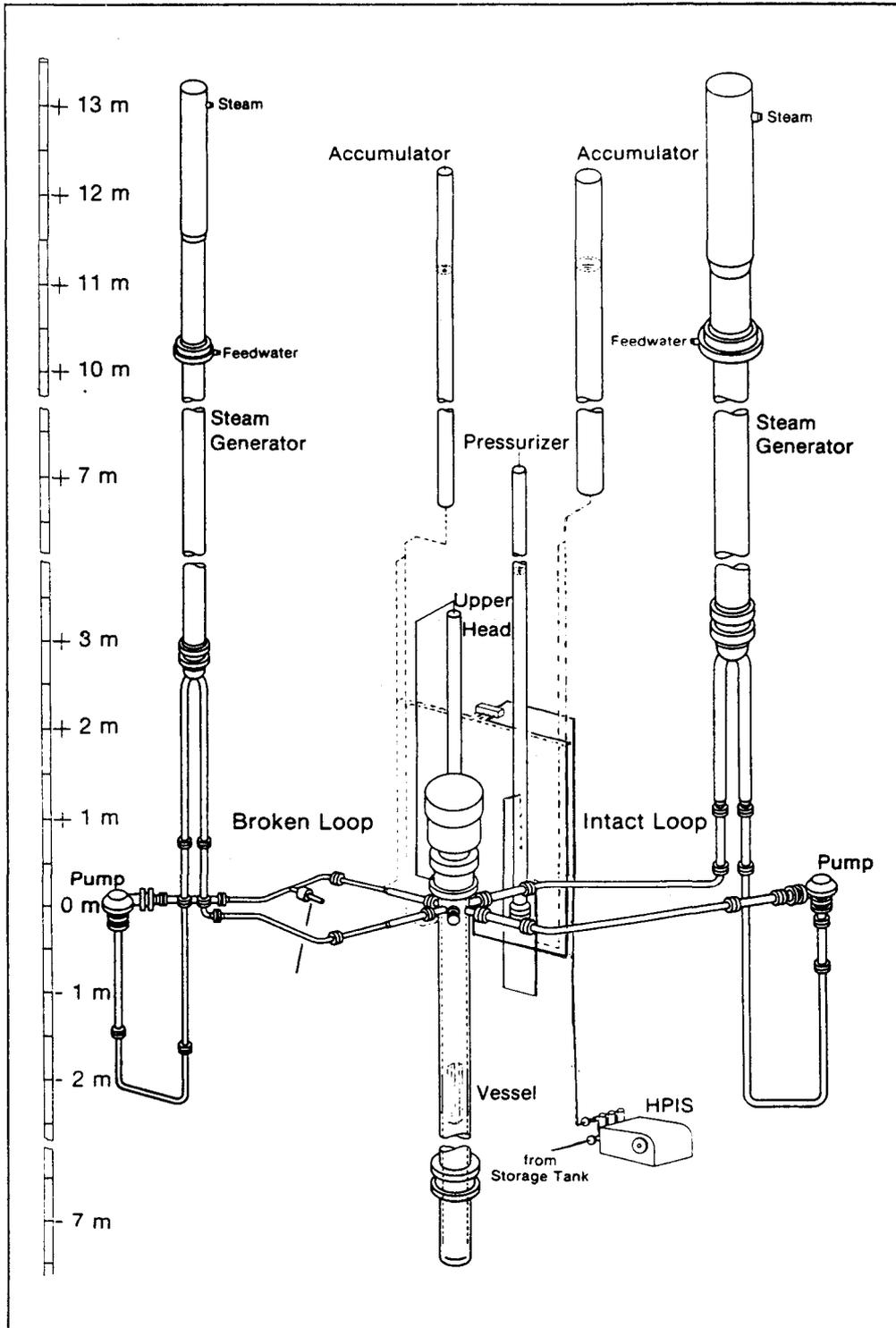
FIG. A.3 LOBI mod.2 Test Facility, primary circuit. Inactive flow lines are shown by dashed lines.
