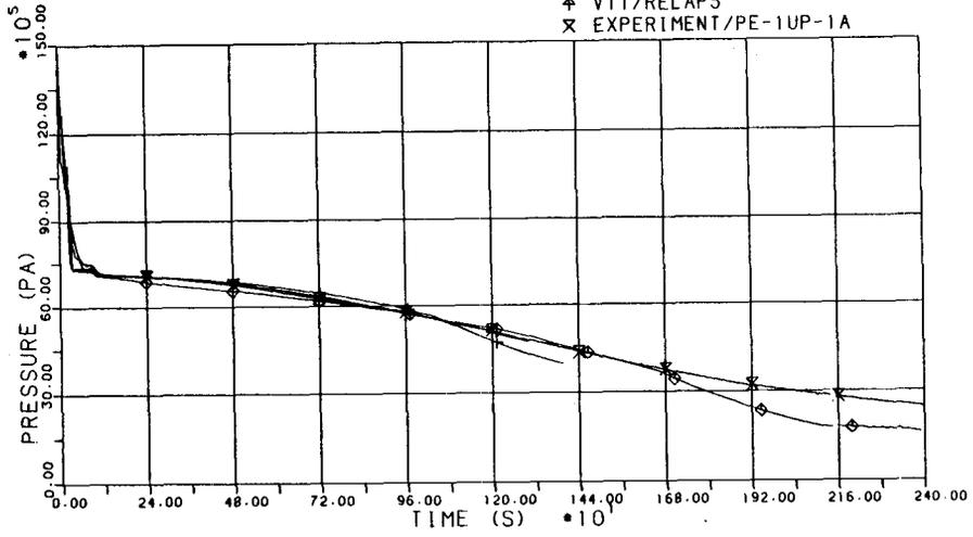
Fig. 3.1.3.1 Pressure in reactor vessel upper plenum
