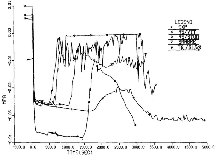
Figure 3.4.6 Differential pressure over descending leg of the loop seal of intact loop.
