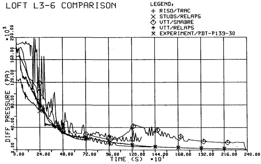
Fig. 3.1.3.4 Differential pressure across reactor vessel
