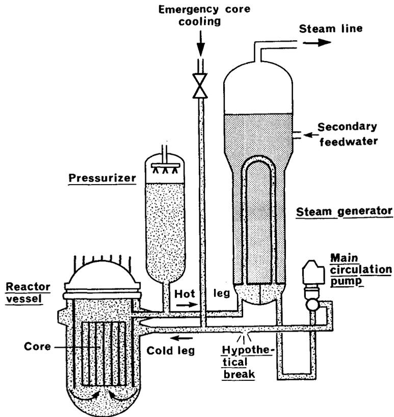
Cover picture: Principal coolant circuit in a pressurized water reactor (PWR).
