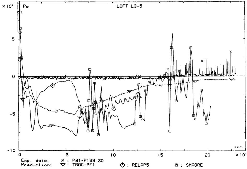
Fig. 3.1.4.5 Different pressure across reactor vessel
