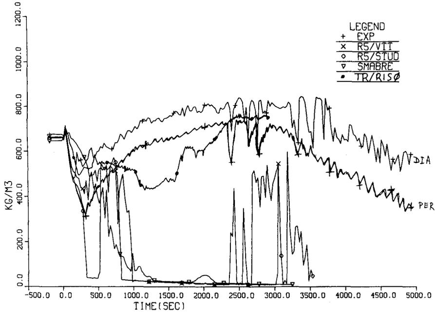
Figure 3.4.4 Mixture density in intact loop hot leg (vessel outlet).
