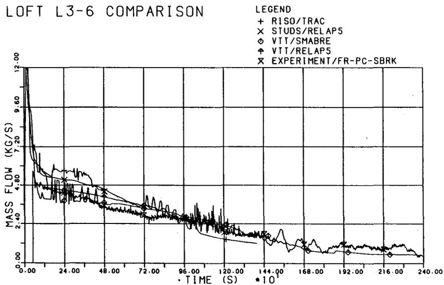
Fig. 3.1.3.6 Break mass flow
