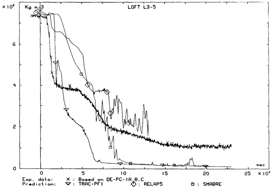
Fig. 3.1.4.4 Mixture density in intact loop cold leg
