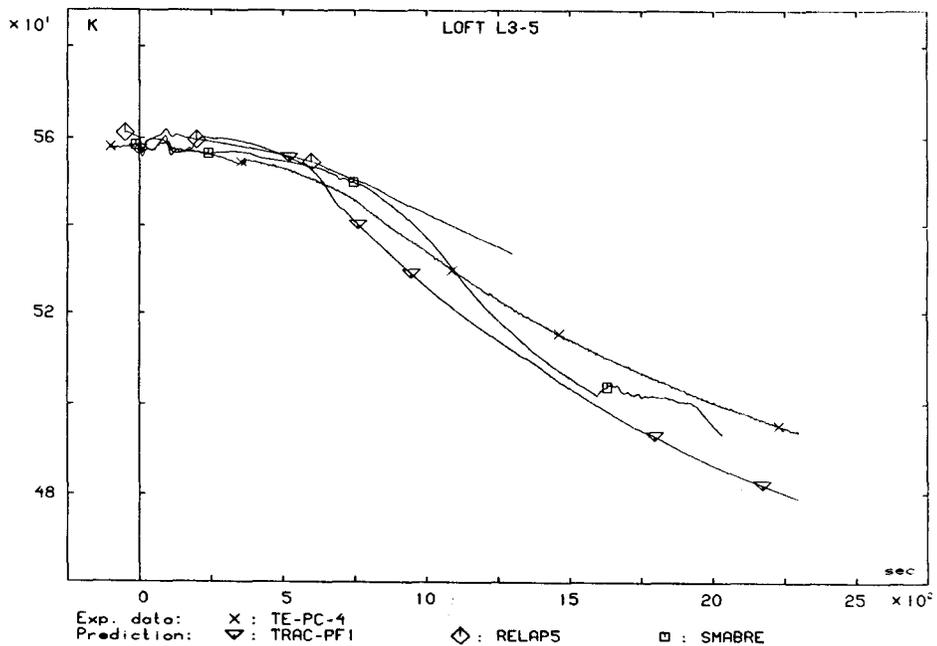
Fig. 3.1.4.2 Fluid temperature in intack loop cold leg
