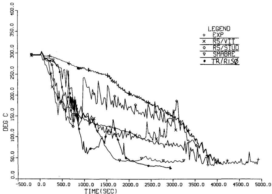
Figure 3.4.3 Fluid temperature intact loop cold leg (vessel inlet).
