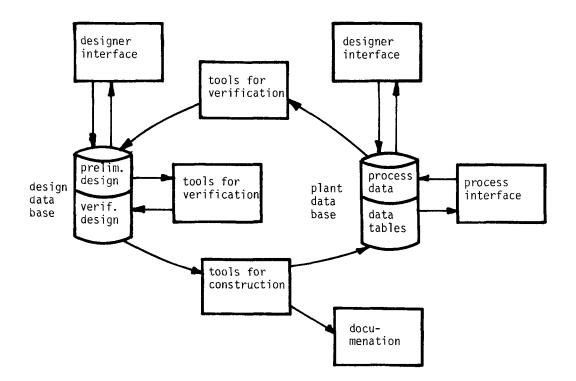
Figure 4.2 The computerized tools of the designer and the operator and their relations to the design data base and the process data base.
