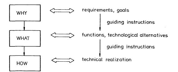
Figure 2.6 The three-level model of the design process.
