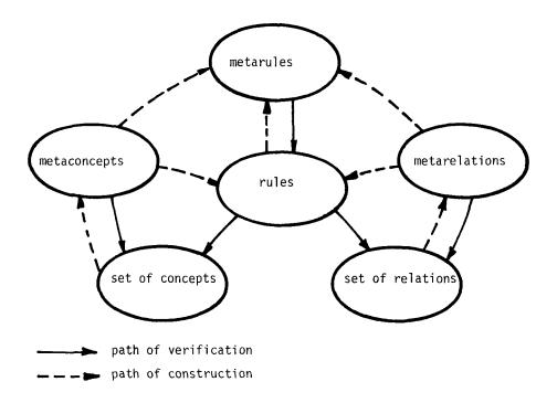
Figure 5.3 The procedure of construction and verification of items in the design data base
