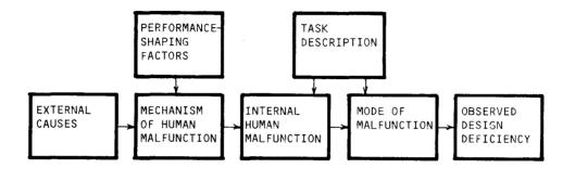
The different boxes in the chain represent different facets of the design errors and can be correlated with each other for an investigation of the most important deficiencies in the design process. The following subdivision of the different boxes is suggested:
