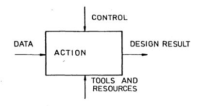
Figure 2.8 A model of the design action, which is used as the building block for the SADT diagrams.
