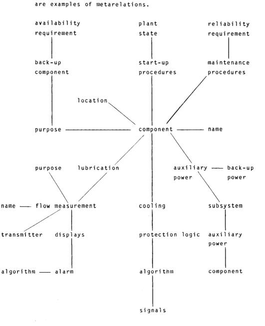
Figure 4.5 Example of possible associations starting from a component. In the design data base it should be possible to move from one object to another along the relations handled.
