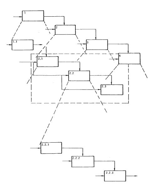
Figure 2.9 The decomposition of the design process.
