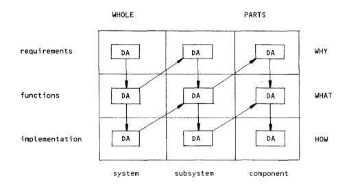
Figure 2.7 The design process broken down with respect to the two dimensions of design. Arrows indicate the temporal ordering between design activities (DA).
