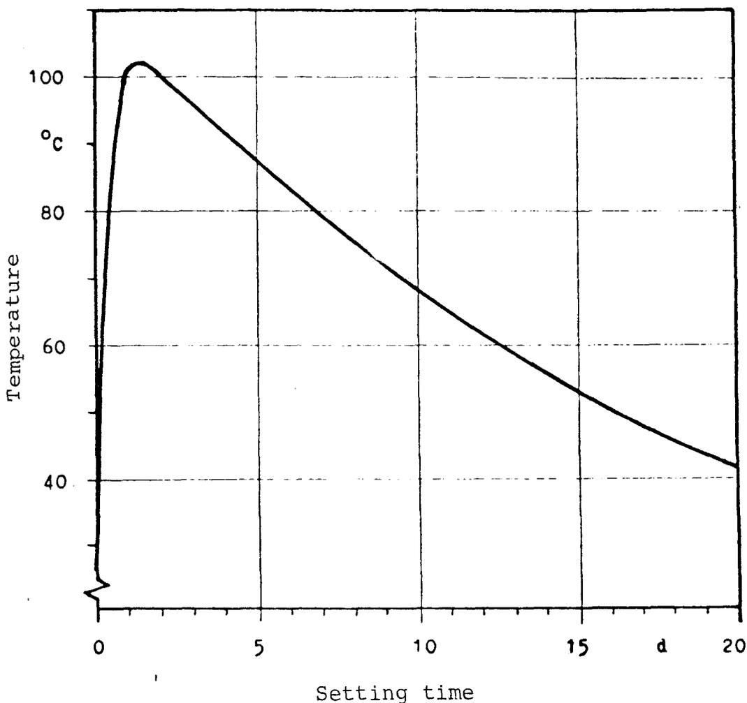
Figure 6.2 Centre-point temperature rise due to heat-generation in styrox (0.5 m) insulated 200 l barrel after pouring Portland Cement  $1025 \text{ kg/m}^3$ , water  $445 \text{ kg/m}^3$ , ion-exchange resin  $260 \text{ kg/m}^3$  or 0.15 dry resin kg/concrete kg /29/.
