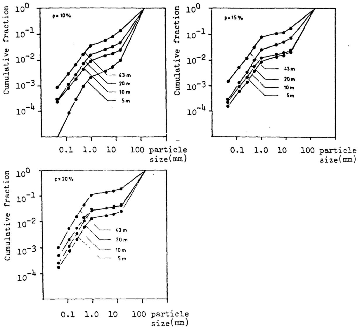
Figure 6.3 Effect of dropping height on the particle size distribution of damaged waste product in different waste mixtures /30/.
