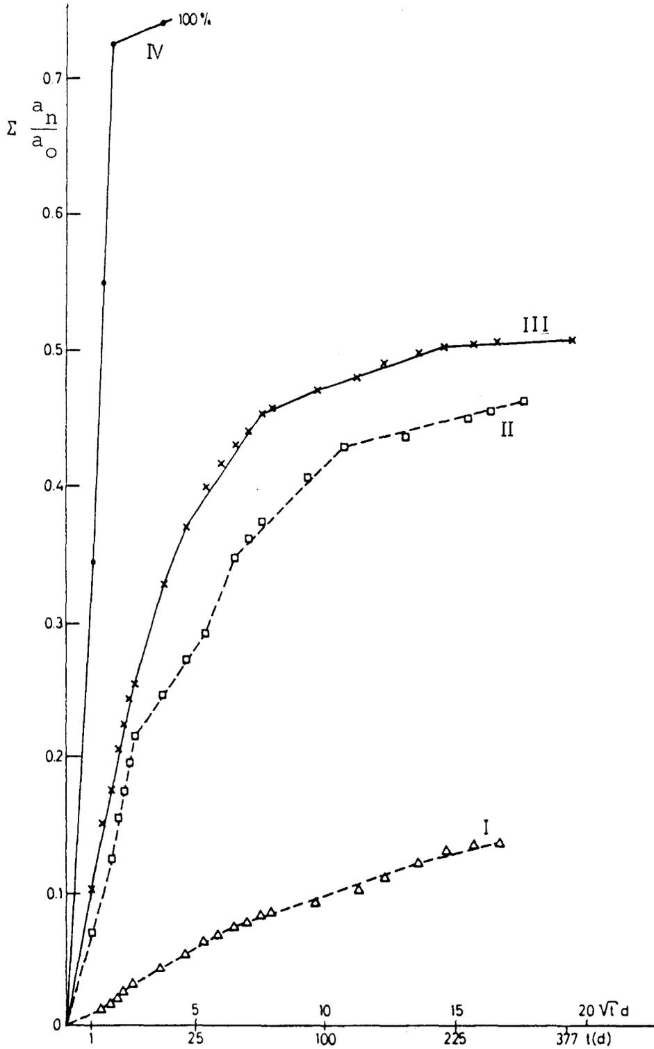
Figure 5.6 Leaching of Cs from crushed and intact cemented ion exchange products, 20% weight % (dry) ion exchange resin.
