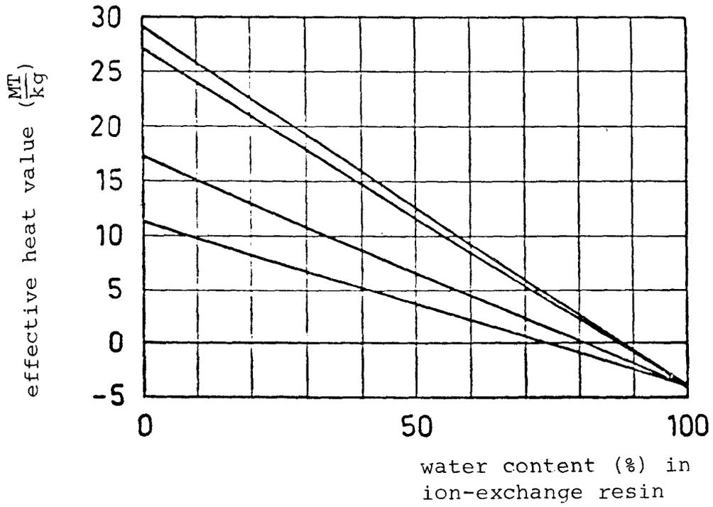
Figure 6.7 Thermal properties for ion-exchange resin/
