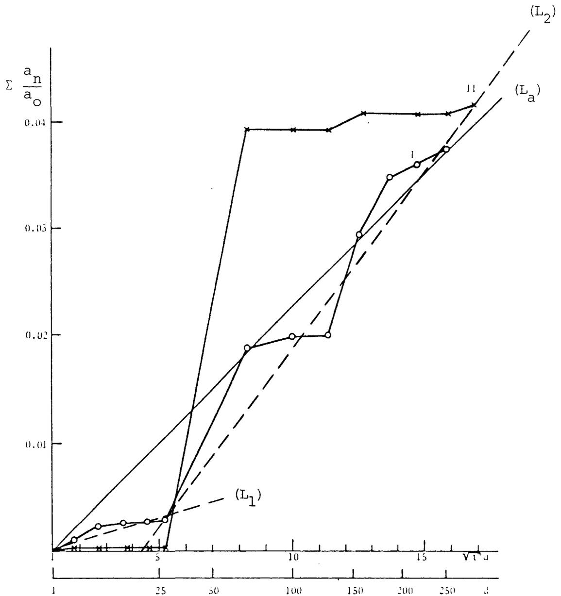
Figure 4.2. Typical stepwise leaching of Cs from ion exchanger-bitumen products in distilled water.
