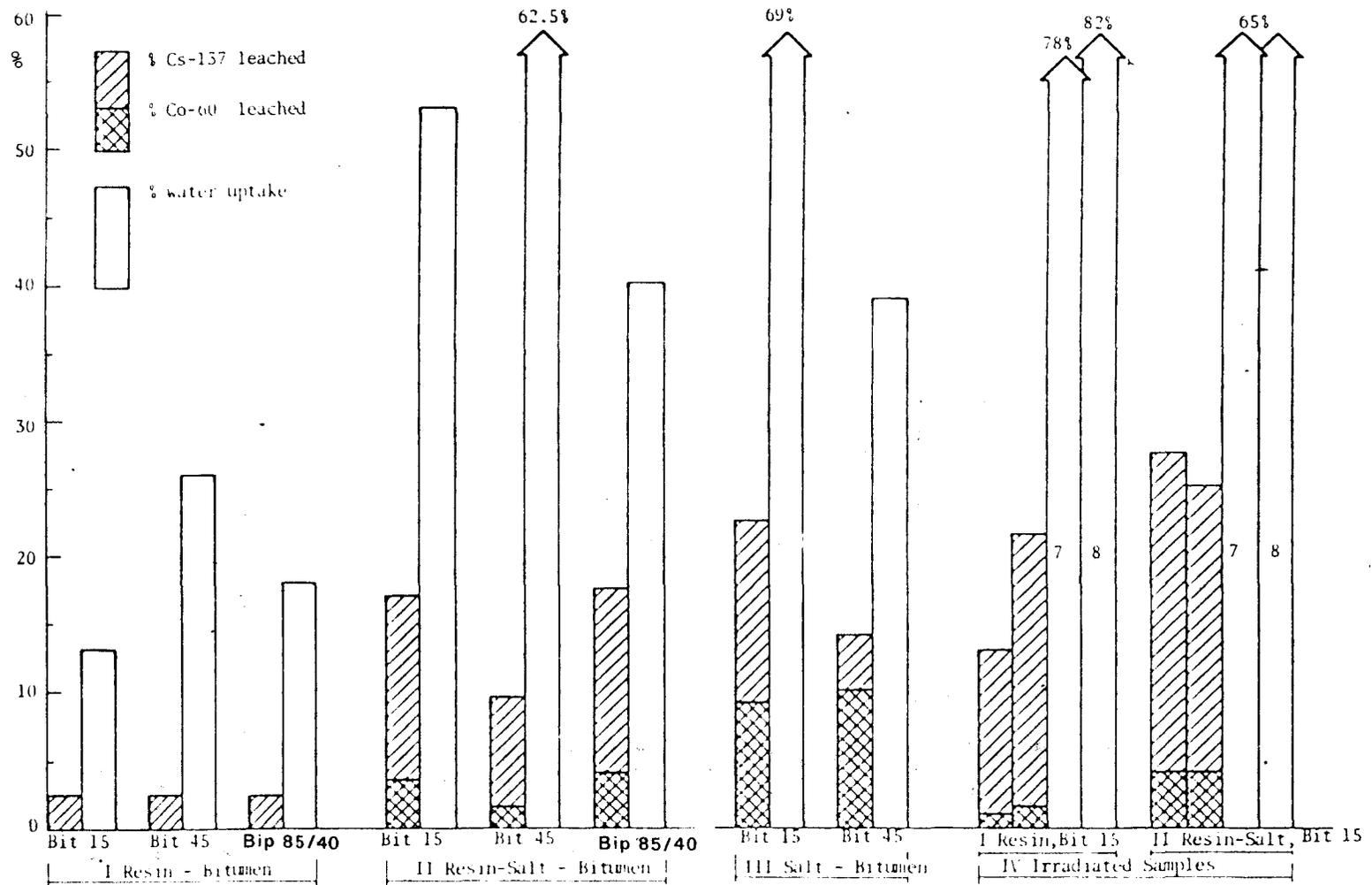
Figure 5.4 Water-uptake, Cs- and Co leaching after 540 days for bitumen products with 40% (40:60 products) of I. ion exchange resin II. resin+salt, III salt. IV. Irradiated samples exposed to  $7/10^7$  and  $8/10^8$  rad.
