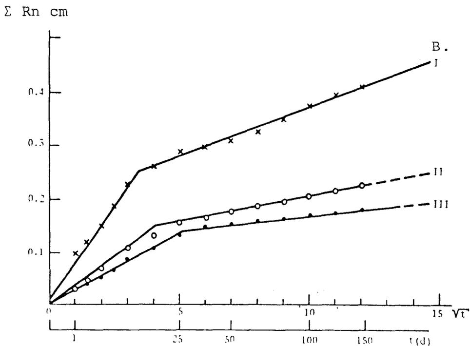
Figure 4.1 Typical leach plots for ion exchanger-cement products.
