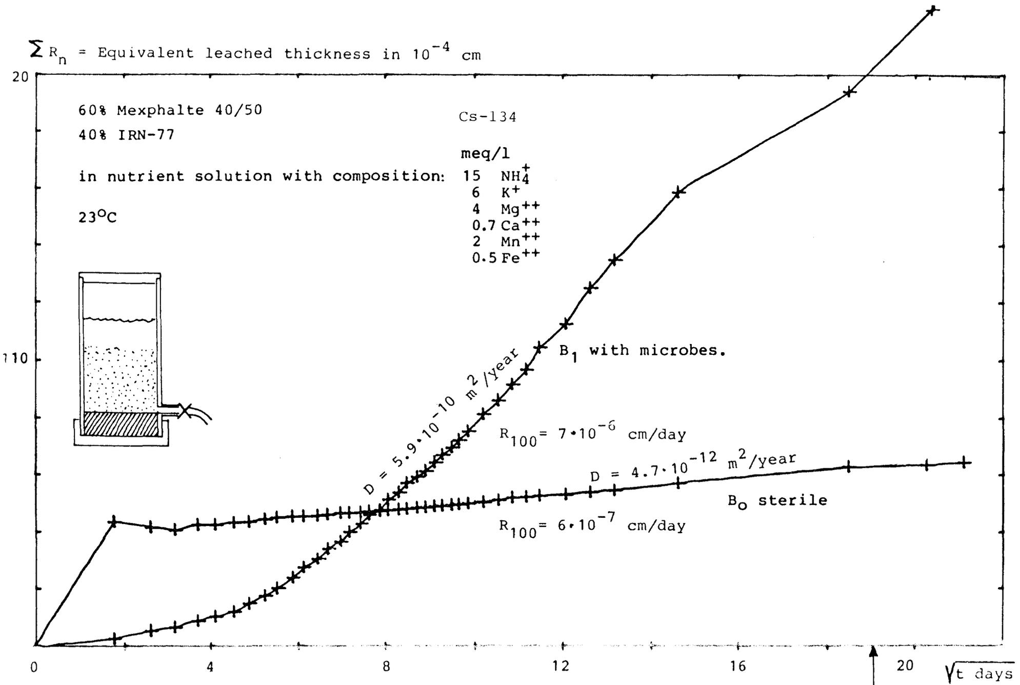
Figure 4.3 Cs-134 leaching in a porous waste system as indicated. With and without microbial growth. (10%)
