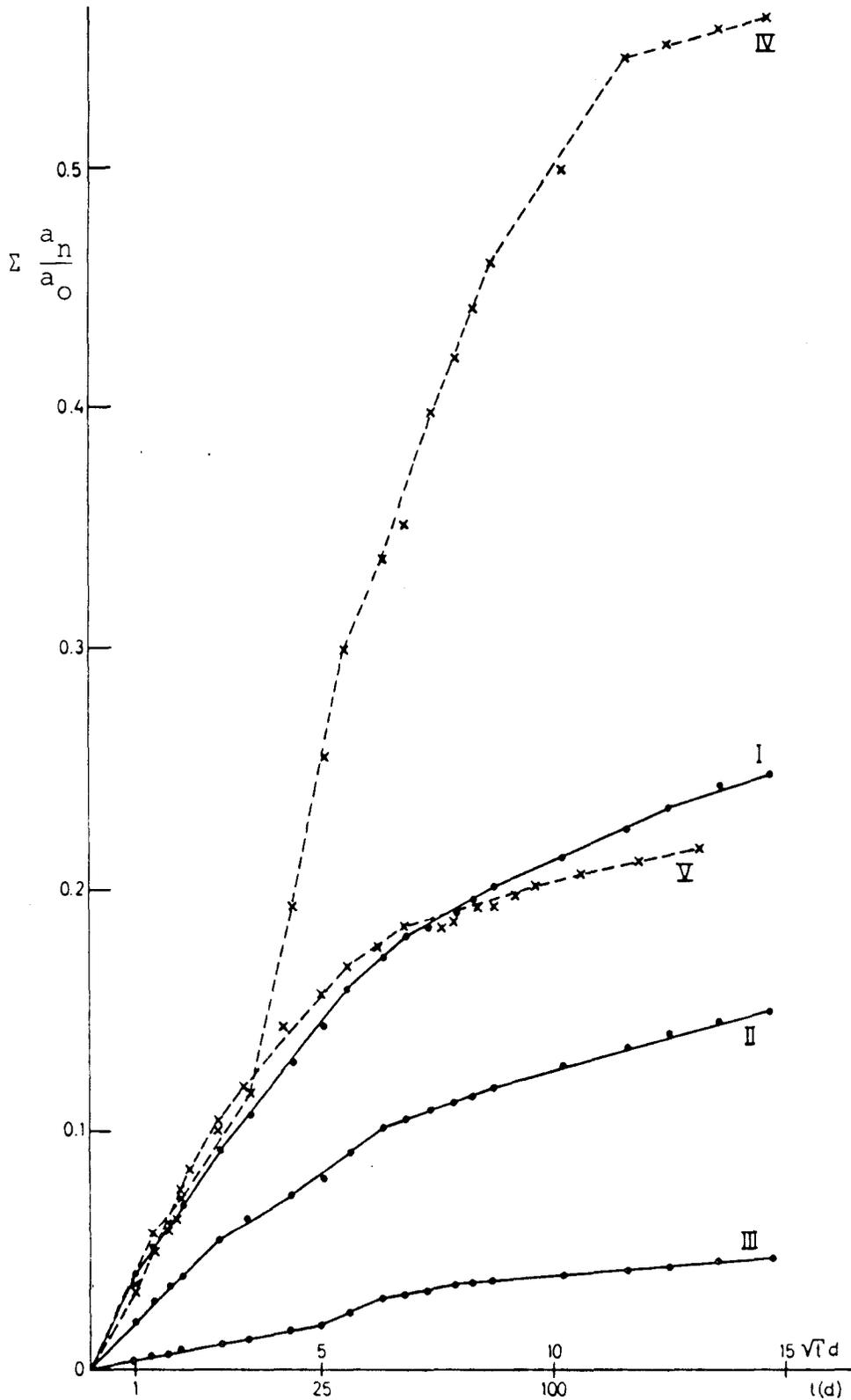
Figure 5.5 Leaching of Cs from slag cement - ion exchange products. Effects of waste loading and stabilizing additives.
