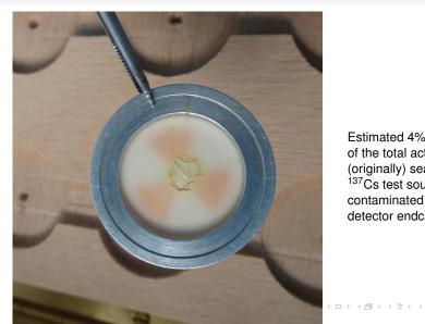
Estimated 4% (7.5 kBq) of the total activity of (originally) sealed <sup>137</sup>Cs test source contaminated the detector endcap.
