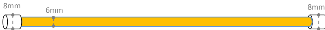
Figure 1: Shape of the source tube (total length = 165 mm) with space for two connectors (diameter = 8 mm, length=10 mm) and the rod radionuclide source (diameter = 6 mm, length = 163 mm).
