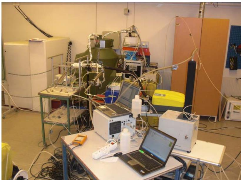
**Figure 2:** An image is presented the experimental set-up for studies on radiolytical oxidation of gaseous methyl iodide by gamma radiation.
