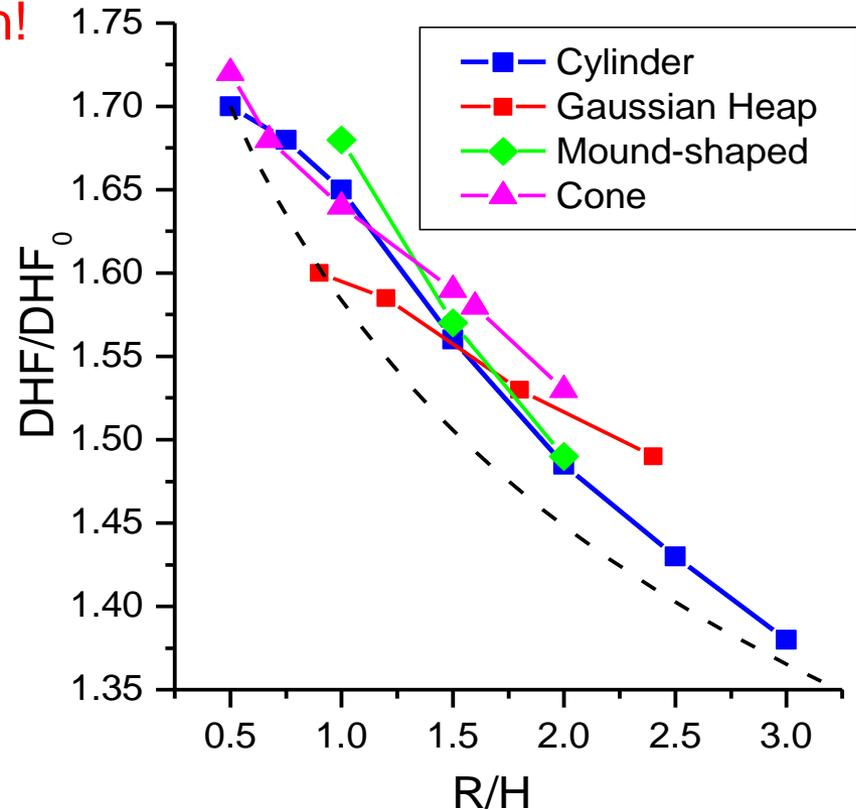
Dependence of DHF on debris bed geometry is factored out.
