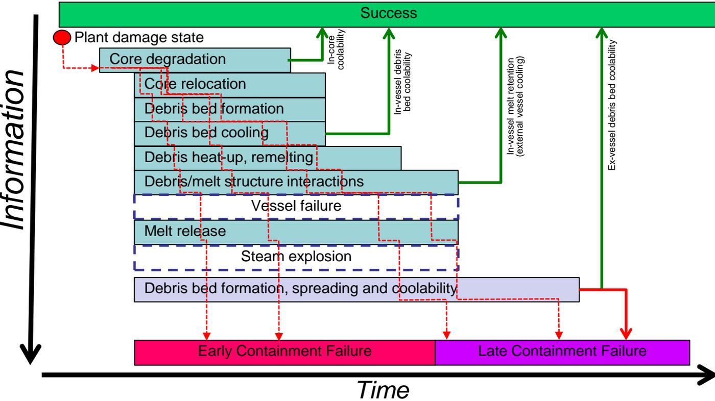
ROAAM+ framework decomposes severe accident progression into a set of causal relationships (CR) represented by respective surrogate models (SM) connected through initial conditions.
