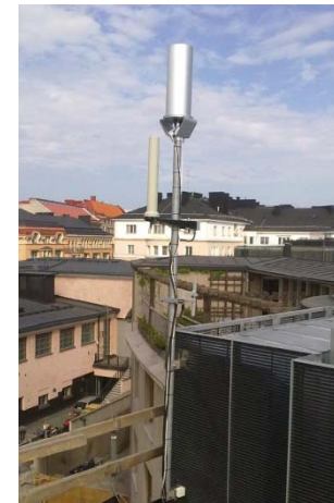
LaBr 3 spectrometer fasten to the lid of the air sampler
